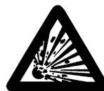
**Standard DRYVAC P pumps are not suited for pumping media which could ignite or explode. If these pumps are nonetheless used in such applications, the owner / operator must take the precautionary measures required for explosion protection in compliance with legal requirements.**
