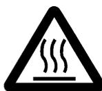
**During operation, the pump’s temperature can exceed 100°C (212°F). Always allow the pump to cool down before removing it from the system or before opening its housing.**
