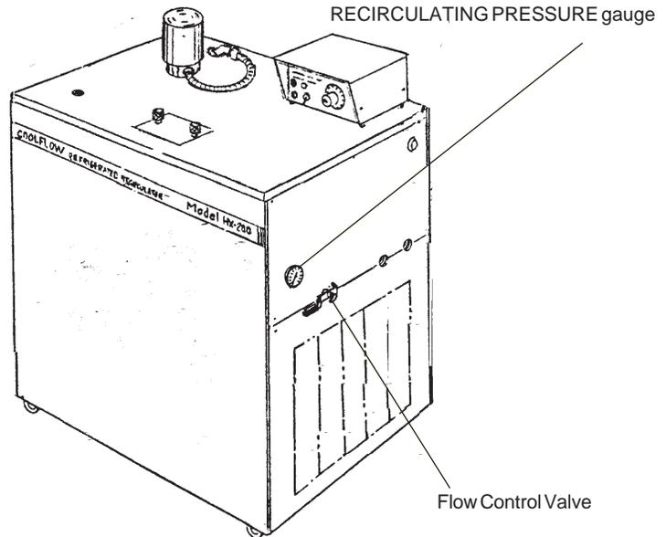
When the handle is in the “+” position, the valve is open and all possible cooling fluid is supplied to the instrument being cooled. When the handle is in the “-” position, the valve is closed and no cooling fluid is supplied to the instrument being cooled. When the handle is between these two positions, the flow rate of the cooling fluid is between full flow and no flow. Use a flow meter on the SUPPLY line to adjust the desired flow rate.
