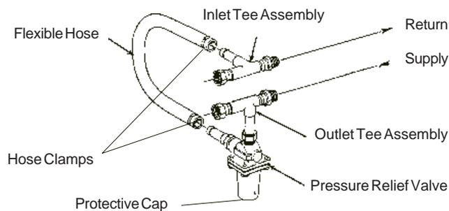
Connect the outlet tee assembly to the inlet of your application. Connect the inlet tee assembly to the outlet of your application.
