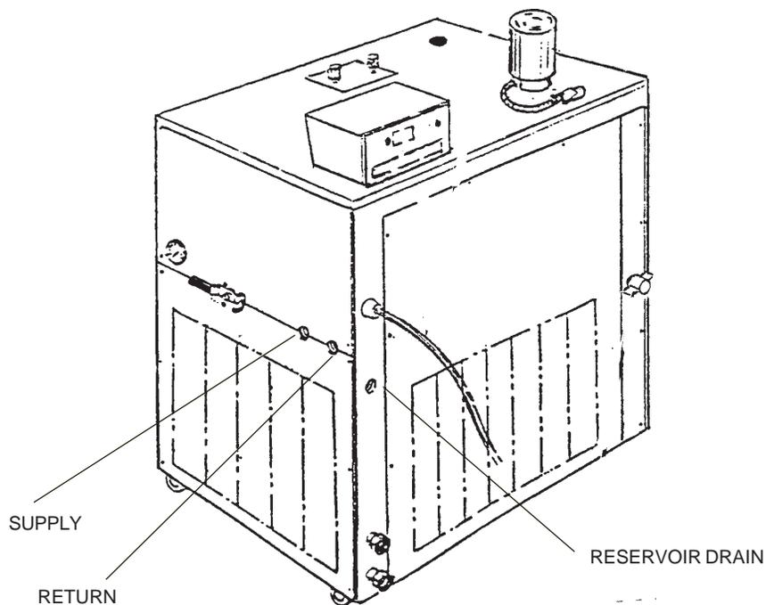
Two plumbing adapters ( $\frac{3}{4}$  inch MPT x  $\frac{5}{8}$  inch hose) are included with the unit. If the unit is being plumbed to the instrument being cooled using flexible tubing, install the adapters in the SUPPLY and RETURN plumbing ports. To prevent leaking, wrap the threads of the adapters with Teflon<sup>®</sup> sealing tape before installing them in the plumbing ports. The adapters will accept  $\frac{1}{2}$  or  $\frac{5}{8}$  inch ID flexible tubing.
