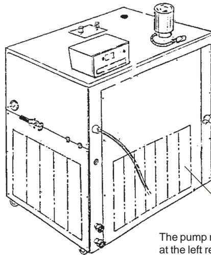
The pump motor overload protector is located at the left rear corner (mounted directly under the fluid reservoir). The fault indicator is visible through the rear access panel.
