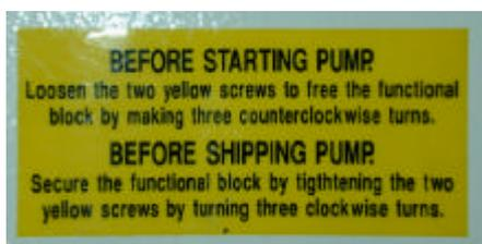
The IPUP A100 pumps are sent from the factory with two screws to hold the functional block in place during shipping.
