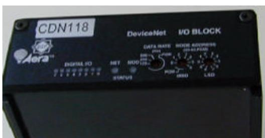
Allows the communication with the equipment by using the Device net protocol.
