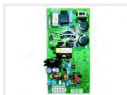
* D001 P0330E1 POWER SUPPLY BOARD - 142/182
