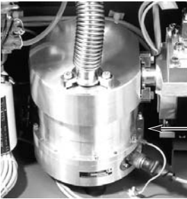
LDS valve (connected to the TMP rear)
