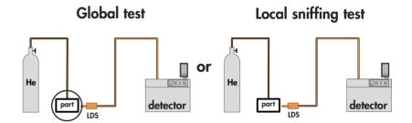
The part is placed under a cover containing a sniffer probe.
