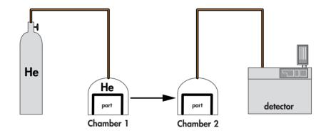
The part is placed in a chamber containing pressurized helium.
