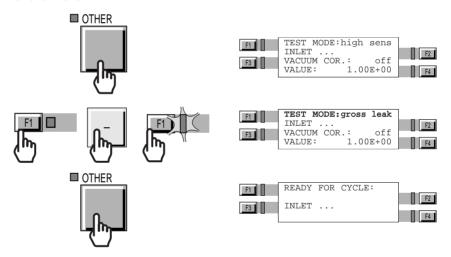
If the leak detector is in gross leak test mode, press 🕅 to go in high sensitivity test mode. The leak detector will switch test mode if the inlet pressure is under the high sensitivity test mode threshold.
