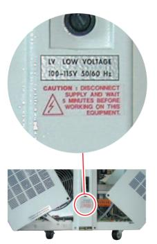
Standard precautions before any maintenance operations: disconnect supply and wait 5 minutes before working on this equipment.
