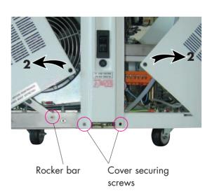
Note: A hinge system is provided on the ASM182 TD+ for the rear cover.
