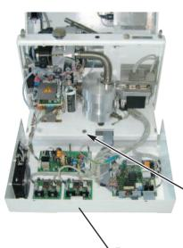
Open the front cover of the detector to be able to access the fourth CHc (allen head) screw securing the stainless steel / I/O interface board assembly. It is located near the hybrid turbo pump (oblong hole on frame).
