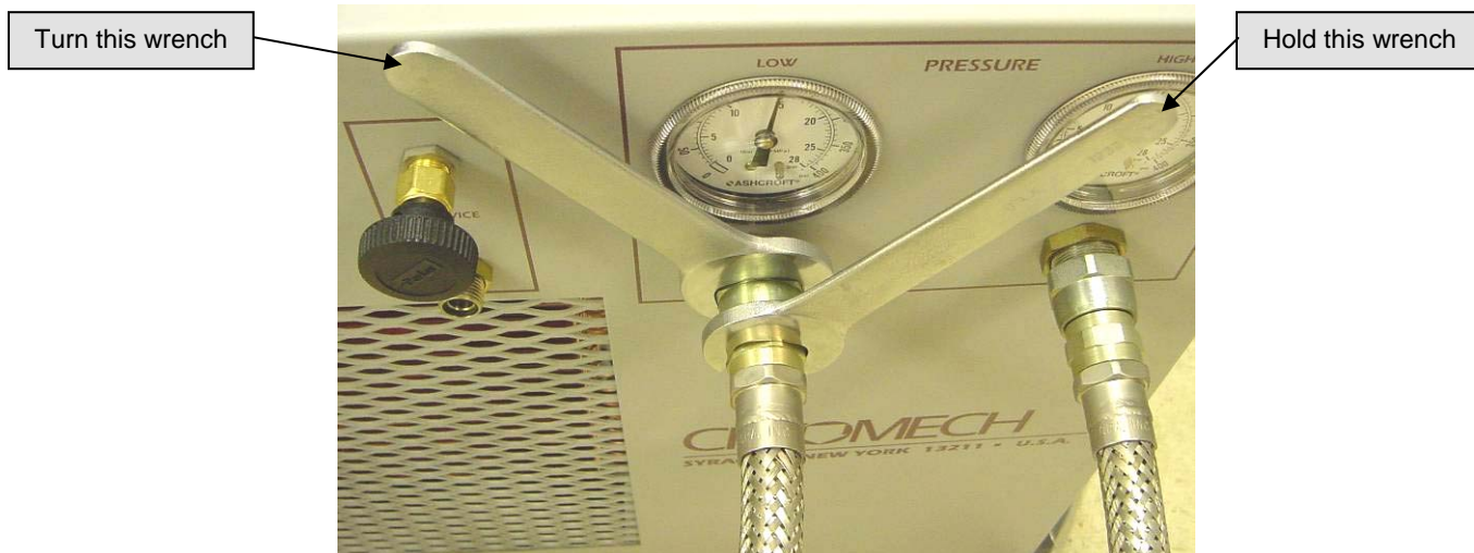
Figure 6-3: Connecting the flex lines to a compressor package
