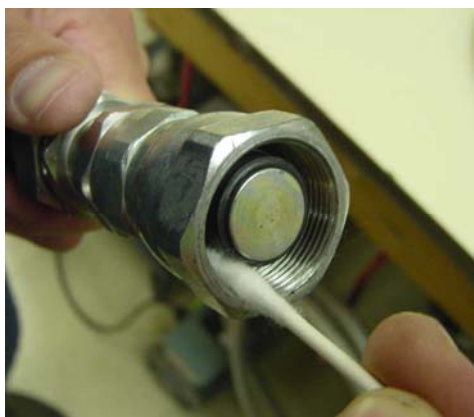
Figure B-1: Cleaning the female Aeroquip
