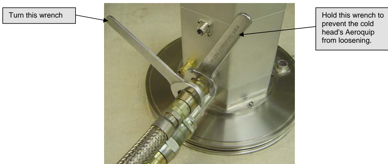
Figure 7-3: Disconnecting flex lines from a cold head
