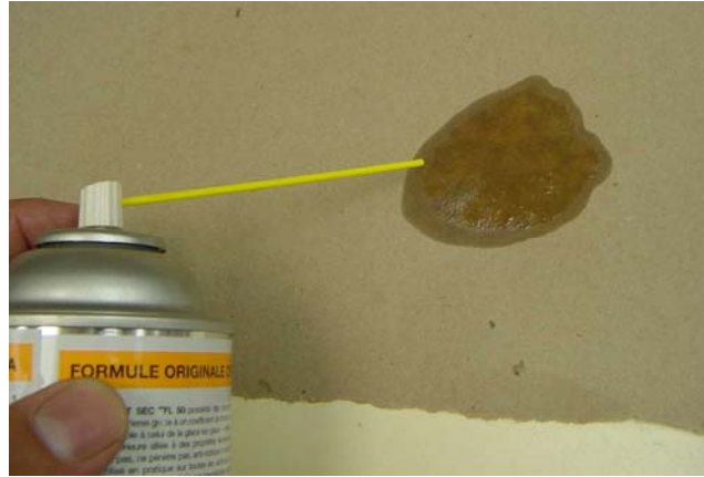
Figure B-4: Typical amount of lubricant
