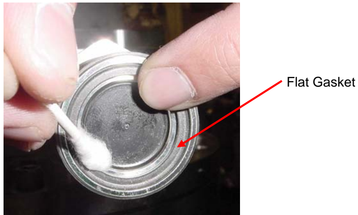
Figure B-2: Cleaning the male Aeroquip®
