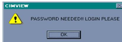
The control system defaults to the last known security level upon startup. The security level can be changed at any time through the Login Panel. The current security level is always displayed as "User ID" at the top left corner of the Overview page.
