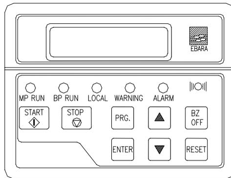
**Fig 6.4 LCD controller**
