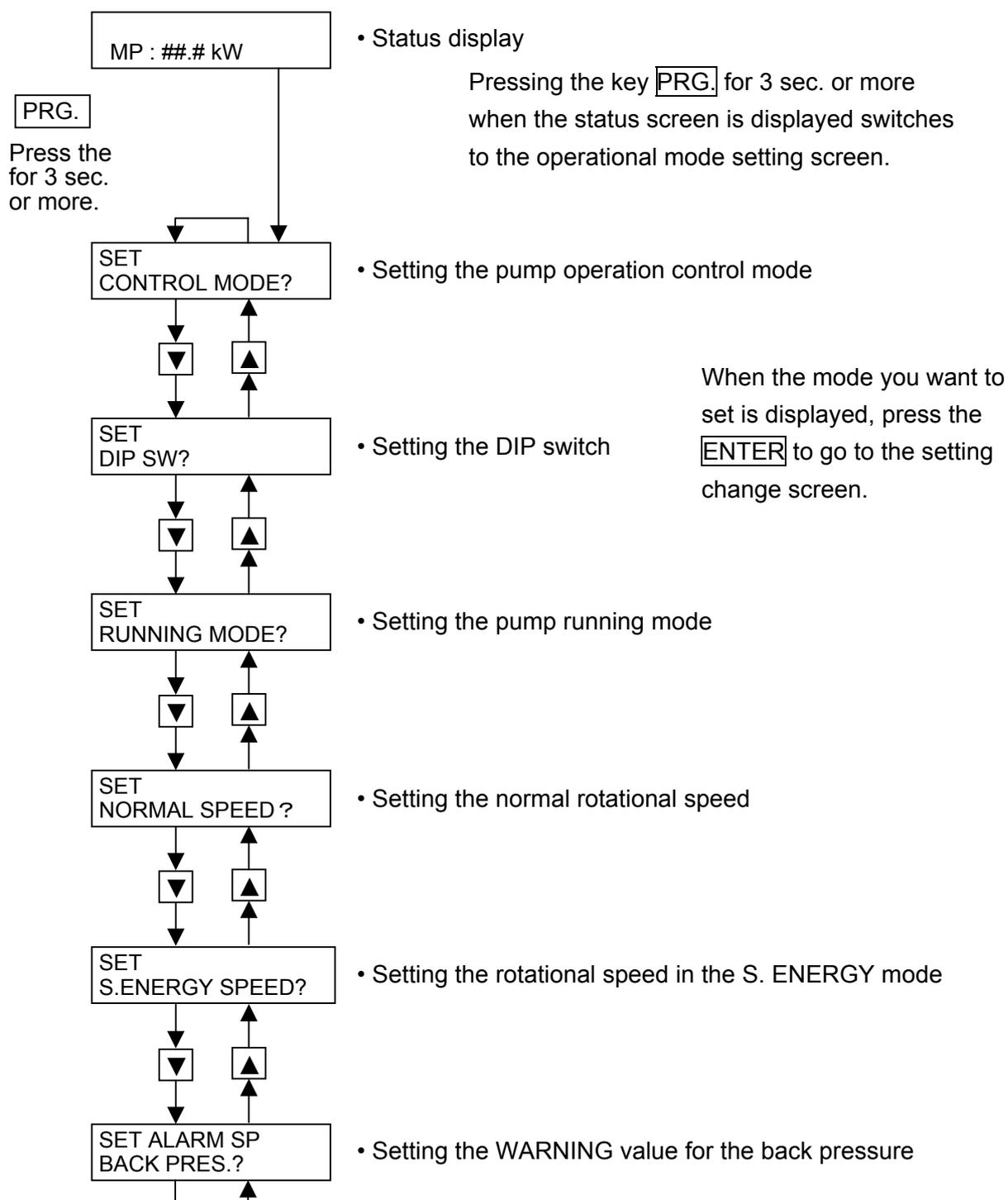
Fig. 6.3 How to set the operational mode
