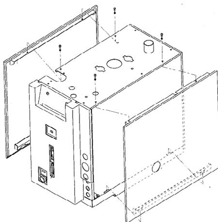
**Fig. 8.1 How to remove pump covers**
