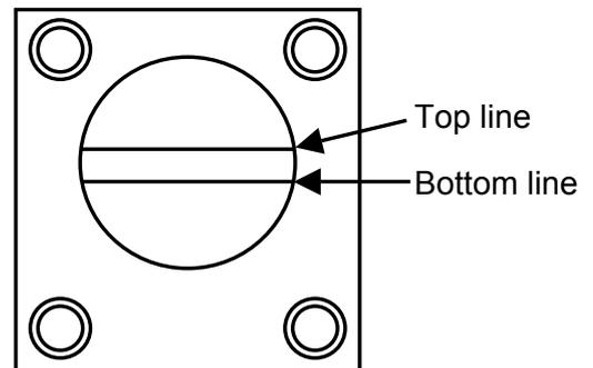
Fig. 8.4 Oil Level Gauge (MP)
