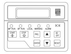
Fig 5.4 LCD controller
