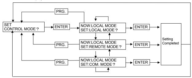
REMOTE MODE: Enables the remote operation
