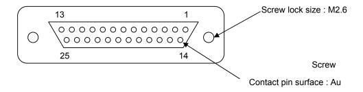
Fig. 3.7 25 Pin D Sub-Miniature Female Receptacle (As seen from connecting side)
