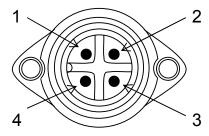
Fig 3.4 Power Supply Receptacle (As seen from connecting side)
