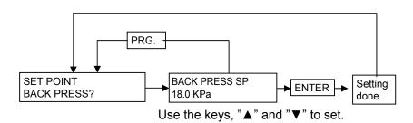
$\triangle$  : Increase the setting speed by 0.5 kPa  $\nabla$  : Decrease the setting speed by 0.5 KPa
