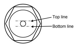
Fig. 7.3 Oil Level Gauge
