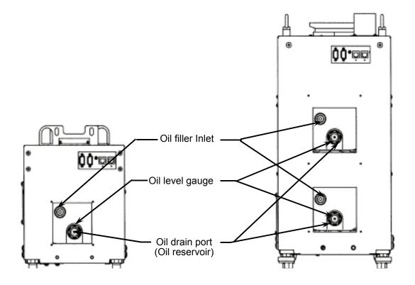
Fig. 7.2 Oil filler inlet, oil level gauge, and oil drain port positions
