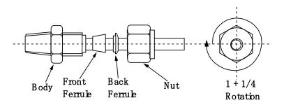
**Tube Fitting Assembly** Fig 3.3
