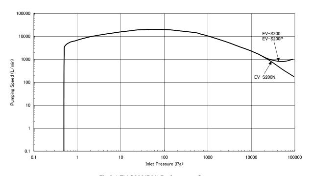
Fig 2.4 EV-S200(P/N) Performance Curve
