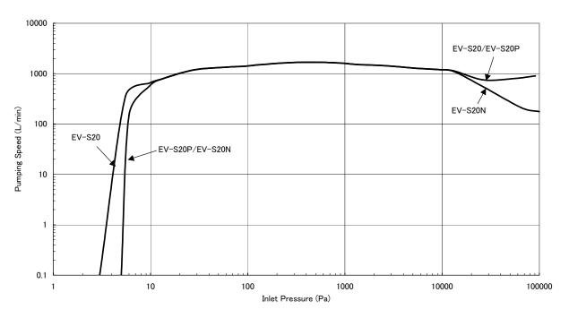
Fig 2.1 EV-S20(P/N) Performance Curve
