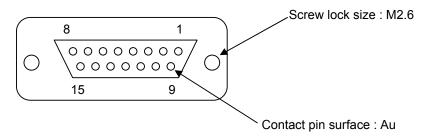
Fig 3.6 15 Pin D Sub-Miniature Female Receptacle (As seen from connecting side)
