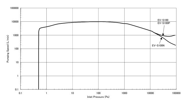
Fig 2.3 EV-S100(P/N) Performance Curve
