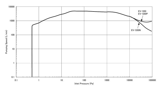
Fig 2.2 EV-S50(P/N) Performance Curve
