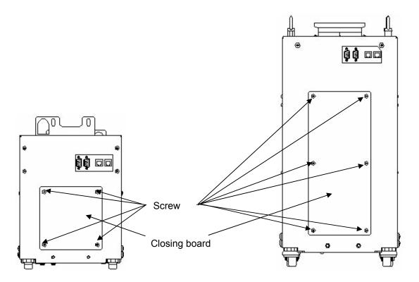
Fig. 7.1 How to remove closing board
