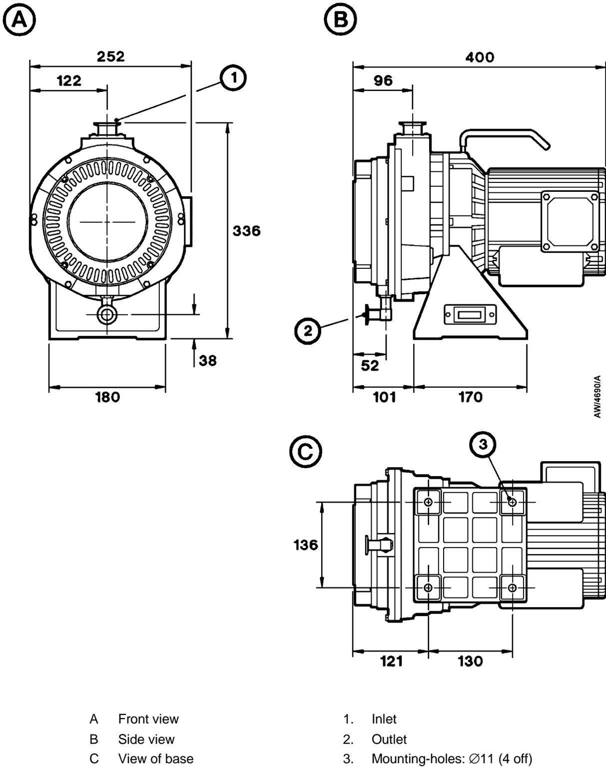
Figure 3 - ESDP12 pump dimensions (mm)
