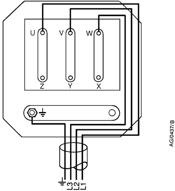
Figure 10 - ESDP30 motor terminal-box low-voltage configuration: 3-phase pumps
