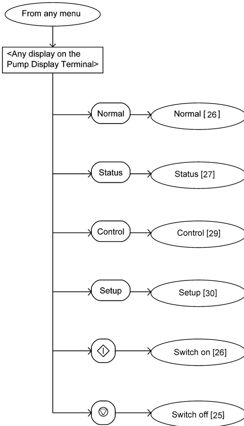
⚠ If the Pump Display Terminal does not have control when you try to switch on or switch off the pumping system, an error message will be displayed: refer to Table 19 .
