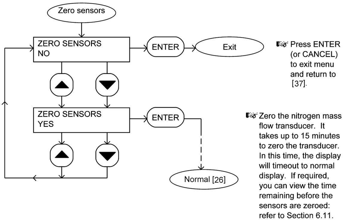
Figure 39 - Gas valve control menu
