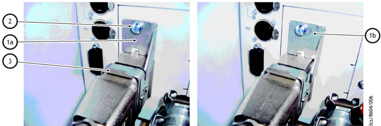
Figure 6 - Electrical connector locking mechanism
