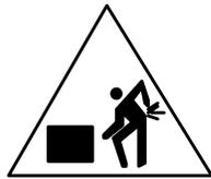
This label is used to caution the user that the unit weighs over 35 lbs (16 kg) and should be moved by two people.
