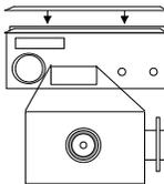
10. Make sure that the unit covers and the RF output cover are on. There are safety interlocks in all these locations that must be engaged or the unit will not work. (See section 2.7 for more information about the safety interlocks.)
