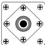
9. Connect the load from the plasma chamber to the RF output connection. This will vary depending upon the application you are using.
