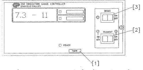
Fig. 1.12 350 IGC Control Unit Front Panel
