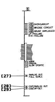
Fig. 5.11 Convectron Module Top View
