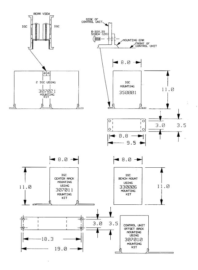
Fig. 1.3 350 Mounting Configurations
