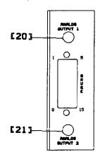
Fig. 5.9 Convectron Module Rear Panel
