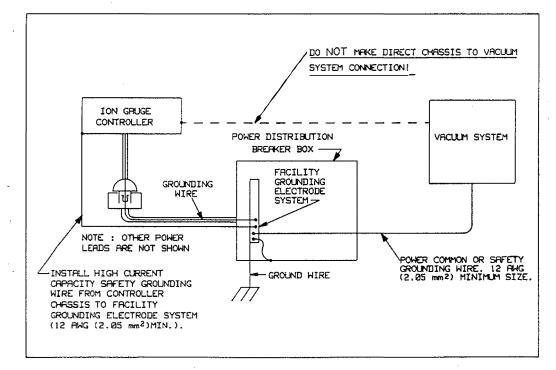
Fig. 1.11 Correct System Grounding
