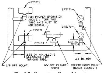
Fig. 5.2 Convectron Gauge Mounting
