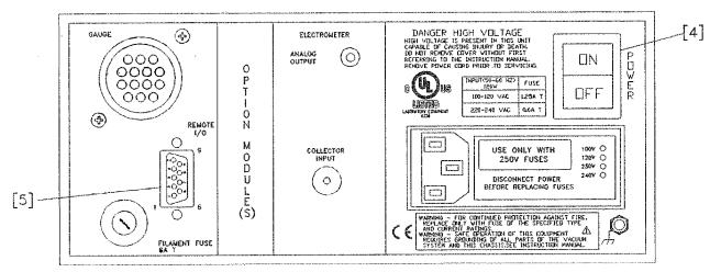
Fig. 1.13 350 IGC Control Unit Rear Panel
