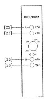
Fig. 5.12 Convectron Module Front Panel
