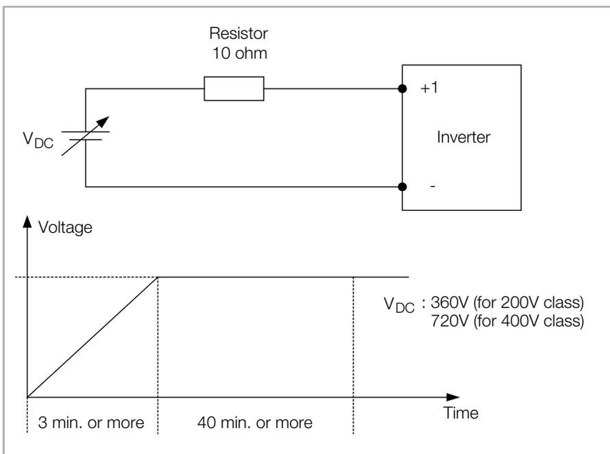
Fig. 2.2 Capacitor forming
