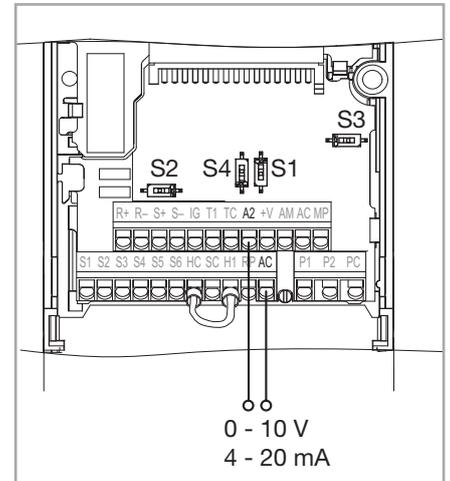
Fig. 4.5 Controlling the speed through a voltage or current input
