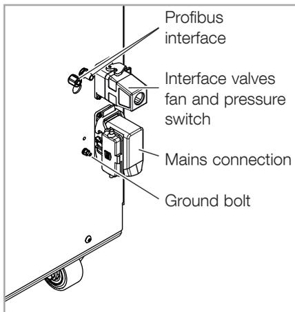
Fig. 3.17 Electrical connections
