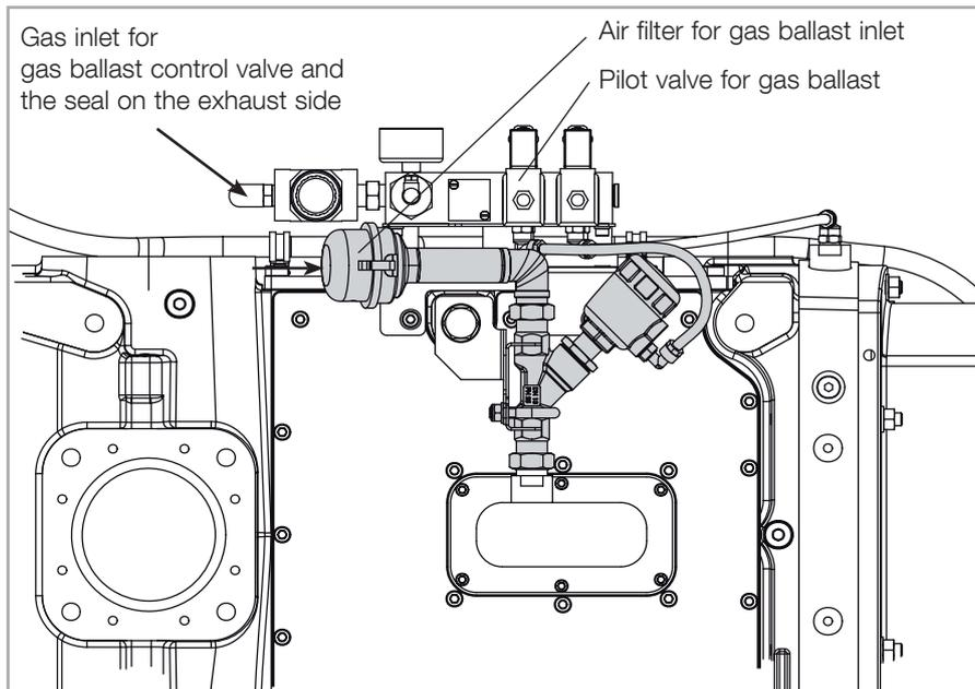
Fig. 3.7 Electropneumatic gas ballast valve (option)
