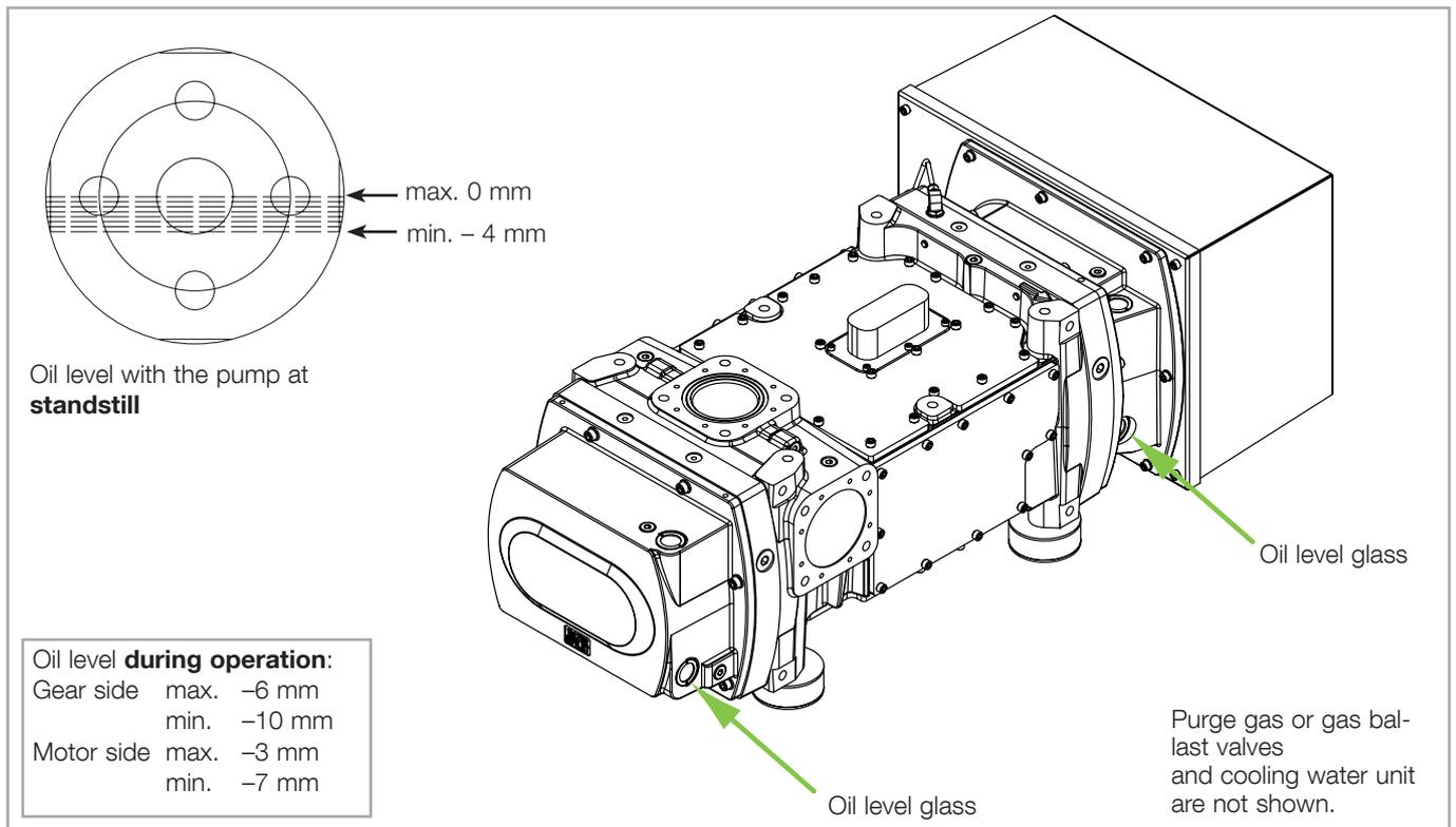
Fig. 3.2 Oil level in the DRYVAC oil glasses
