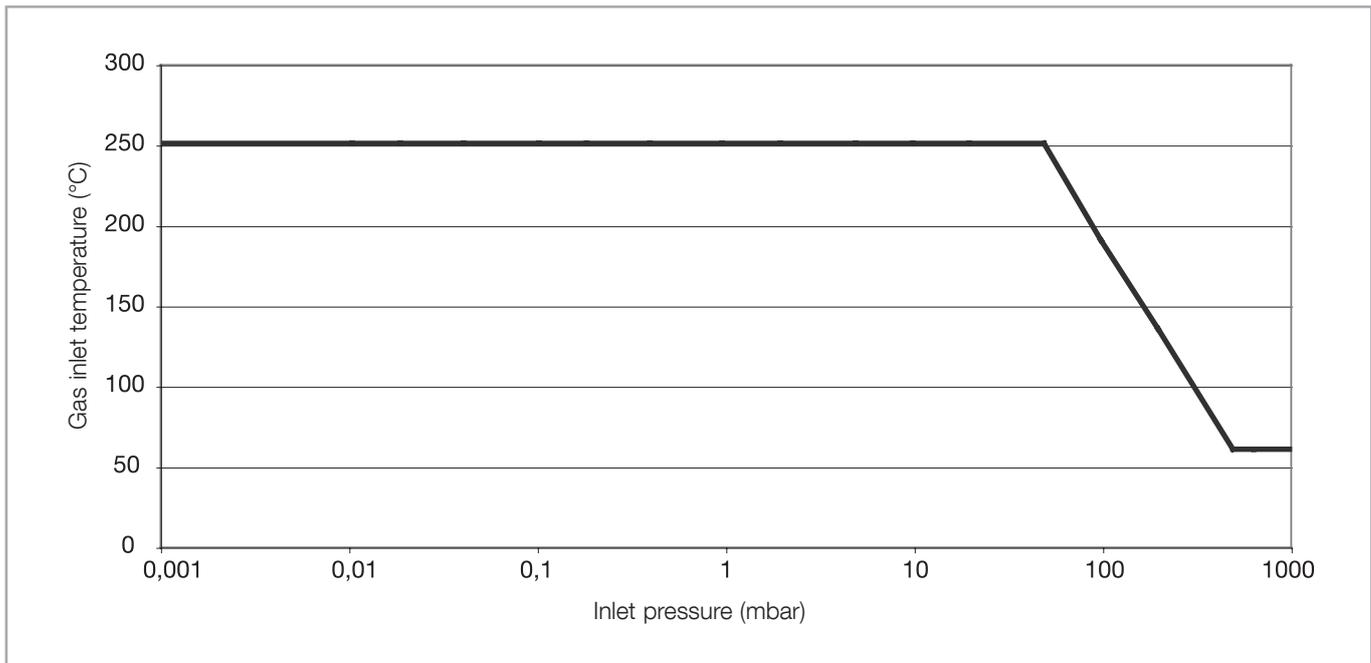
Fig. 1.9 Permissible gas inlet temperature as function of the inlet pressure
