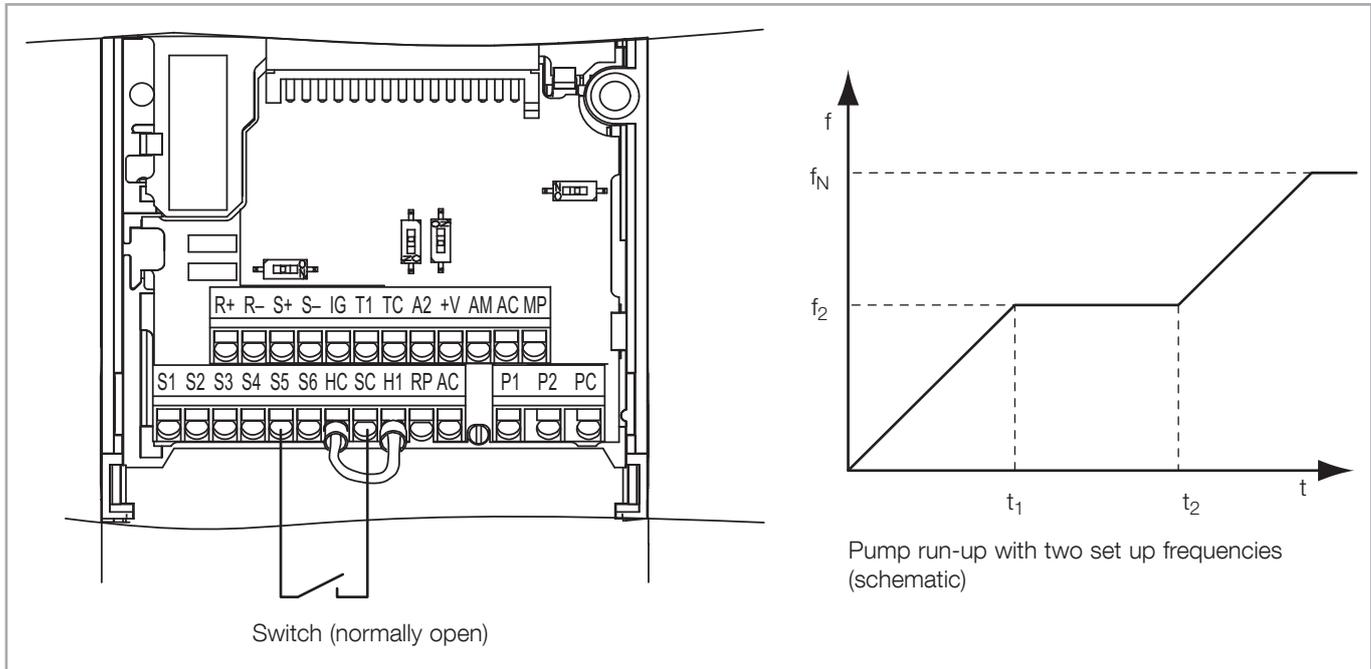
Fig. 4.4 Setting up the second set point frequency
