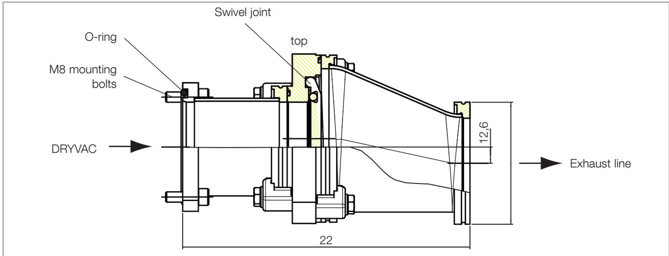
Fig. 3.23 Side view/sectional view of the non-return valve
