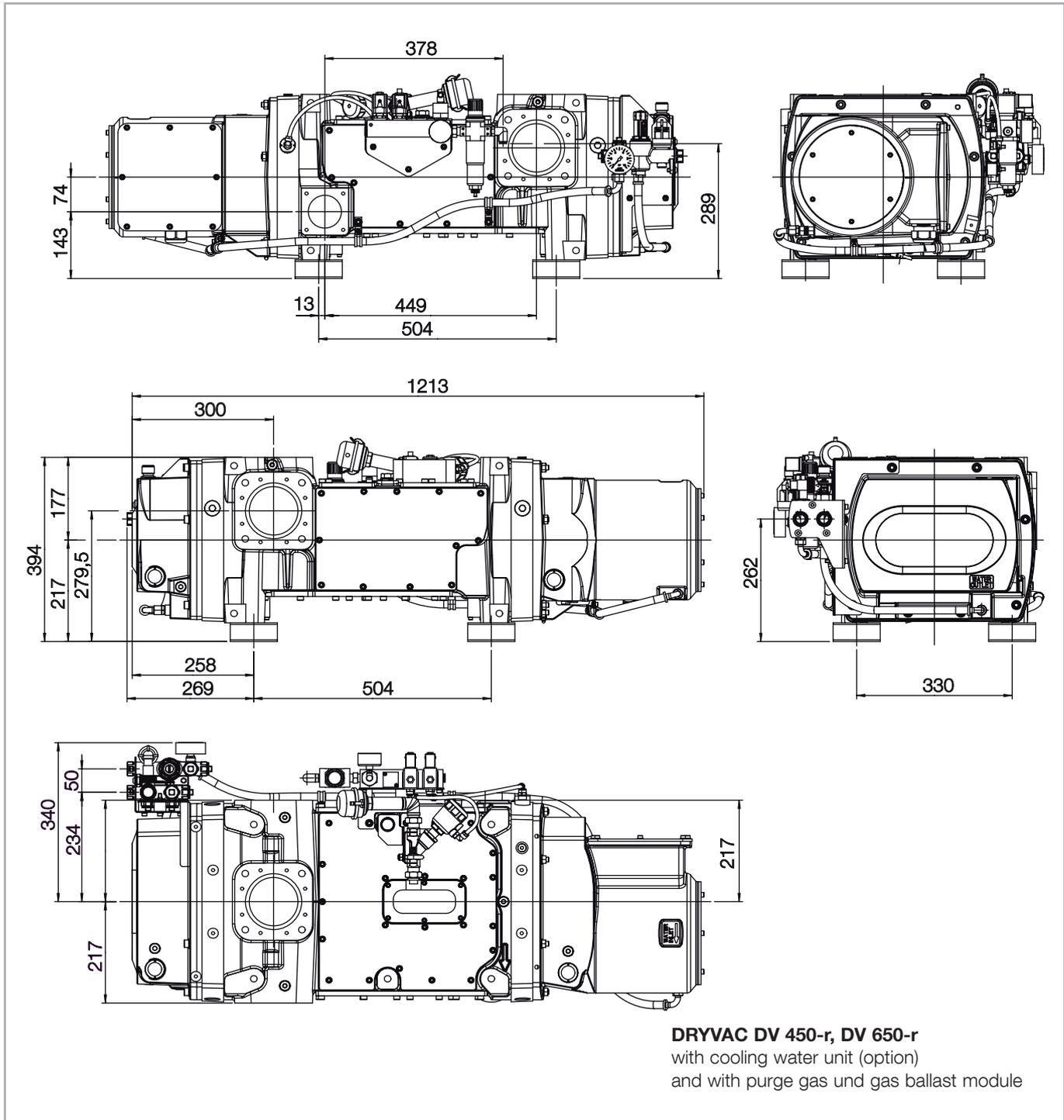
Fig. 1.7 Dimensional drawing, dimensions in mm
