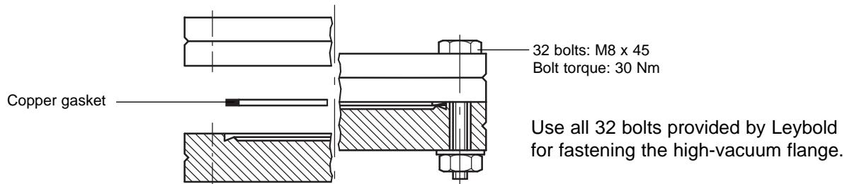
Fig. 2 Section through a CF flange connection
