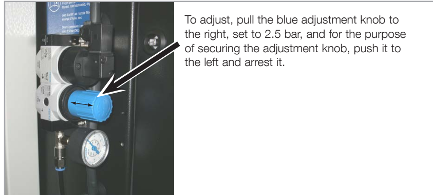
Fig. 4.5 Adjust the pressure reducer
