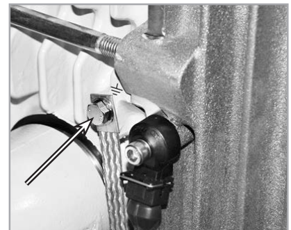
Connect ground strap here!
