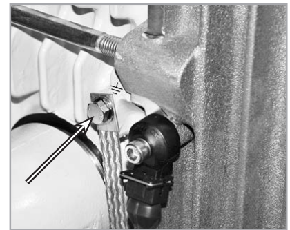
Fig. 3.6 Ground connection example
