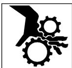
**Caution** The loosened deposits must not remain in the pump. After cleaning, check the pump by slowly turning the impellers by hand. They should move freely and without any resistance.
