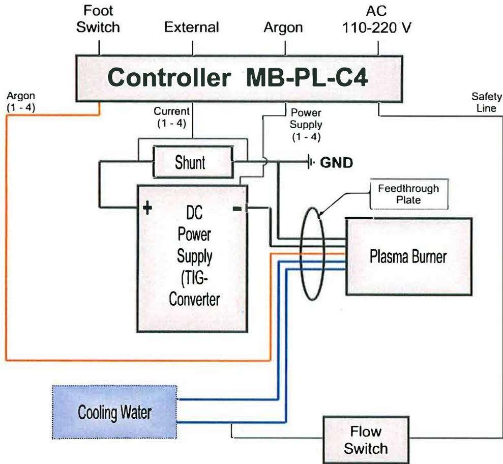
Fig. 9: Plasma Burner System Schematic
