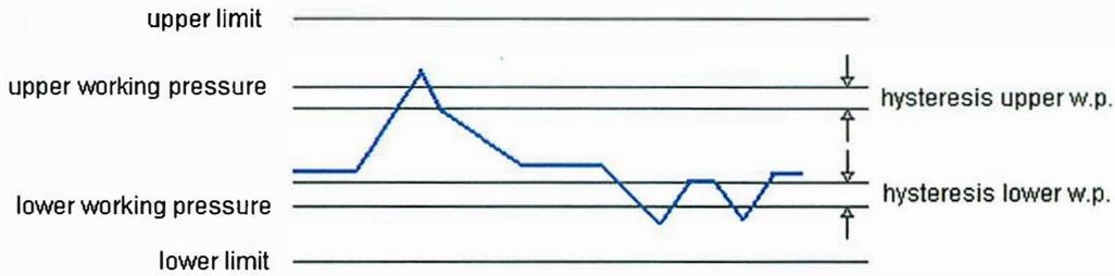
The alarm limits can only be altered in the "Parameter Service" screen.
