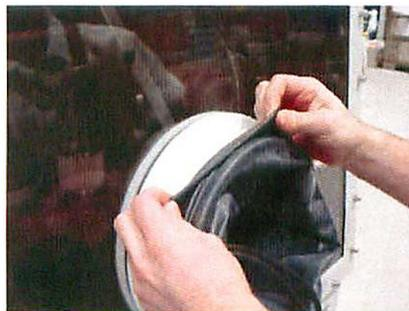
To replace the glove - place the glove over the port so that the rim of the glove locates in the port's innermost groove (the outer 2 grooves are for locating the O-rings that secure the glove).
