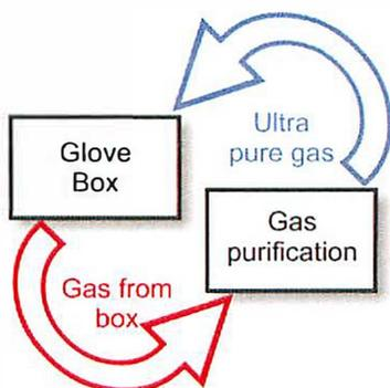
**MBRAUN** systems work by the principle of gas circulation, i.e. the working gas permanently circulates between the glove box and the H<sub>2</sub>O/O<sub>2</sub> gas purification system. This process guarantees absolutely stable values of gas purity and cost-efficient processing.
