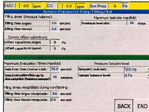
Service Pump filling unit parameters
