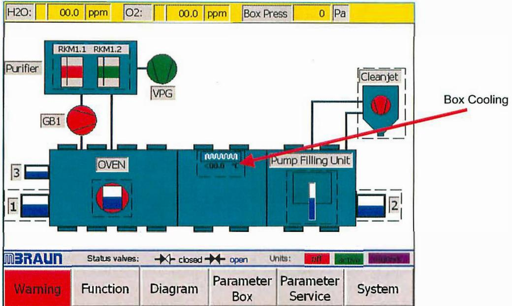
The current temperature of the box is displayed in the centre of the startscreen. By touching the area, indicated above, the Box Cooling Parameters screen is opened.
