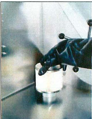
Screw new dust filter in place.
