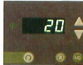
To display the other parameters press the menu/display key. By pressing the key the display cycles through the values for set/low/high/actual temperature
