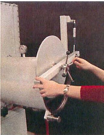
Carefully open the antechamber door in upward direction.
