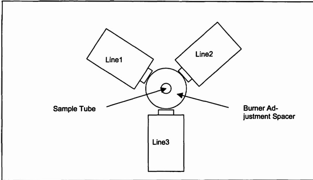
Fig. 16 : Alignment of 3-torch system
