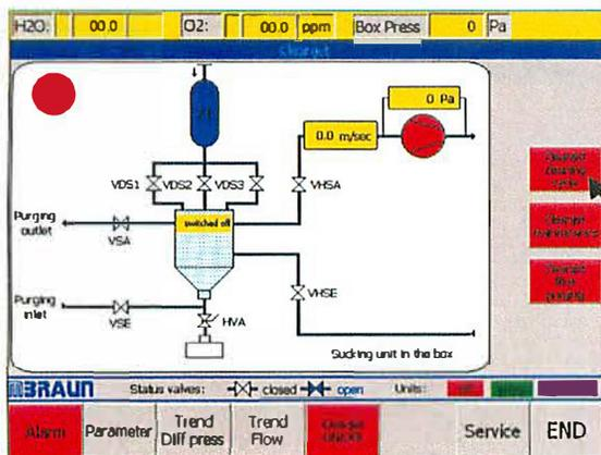
When the filter is exhausted there would be an increase in the differential pressure over the filter. If this difference pressure exceeds the setpoint "Maximum pressure filter" a warning will be given on the Alarm/Warning Screen. This warning will indicate that the filter may require a cleaning process.
