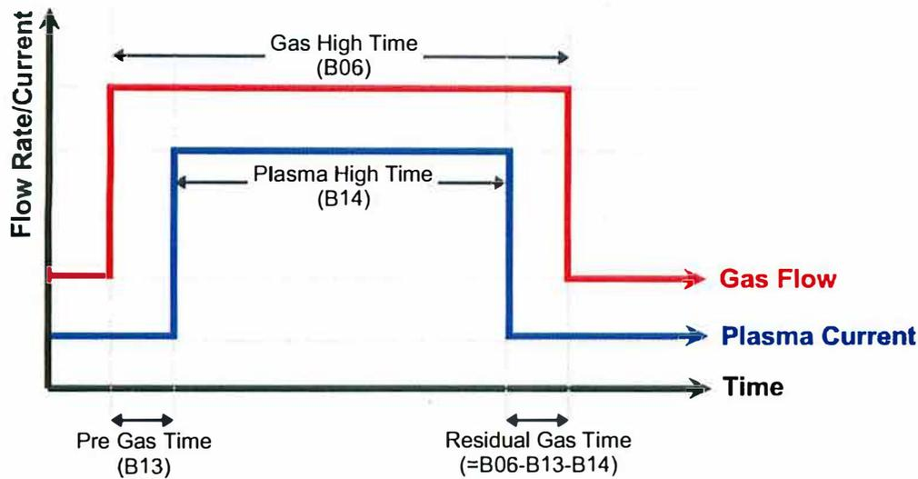
Fig. 10 : Plasma Controller automatic mode timing
