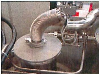
Leave the pipe open for at least 2 minutes to allow the excess Oxygen flow out of the pipe.
