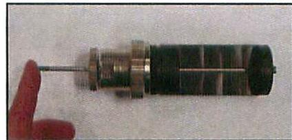
The cathode assembly is now properly adjusted and ready to be mounted on the plasma burner by just inserting the Tungsten rod and fastening the large knurled screw.
