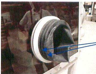
The Gloves are secured by two O-rings.
