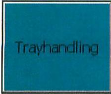
With this button, in the "Oven process screen" you can select the "Trayhandling screen". In the "Trayhandling" screen all the loading and unloading functions for the oven are available.
