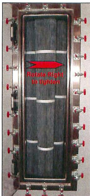
Clean the Door Seal with lint free cloth and lightly smear with high vacuum grease.
