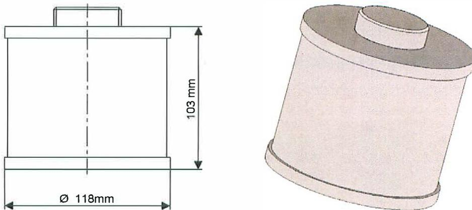
The standard filter is of a HEPA format (class H14)- i.e. filtering 99.995% of particles – typically down to 0.2 microns.
