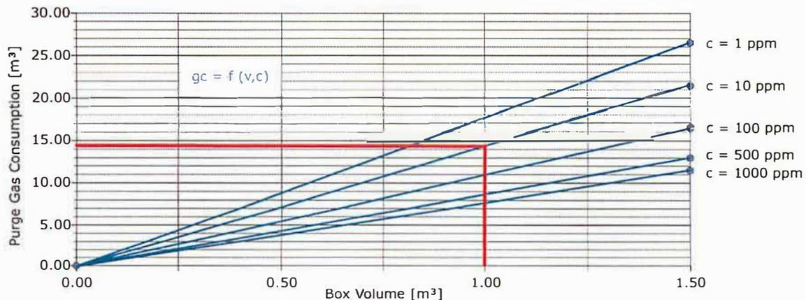
In the example, it shows that if a purity of 10 ppm is required, then about 14.50m<sup>3</sup> of purge gas is required for 1 m<sup>3</sup> box volume.
