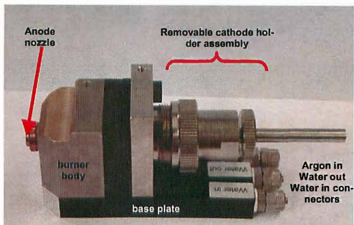
Fig. 12 : Plasma Burner MB-PL-B1
