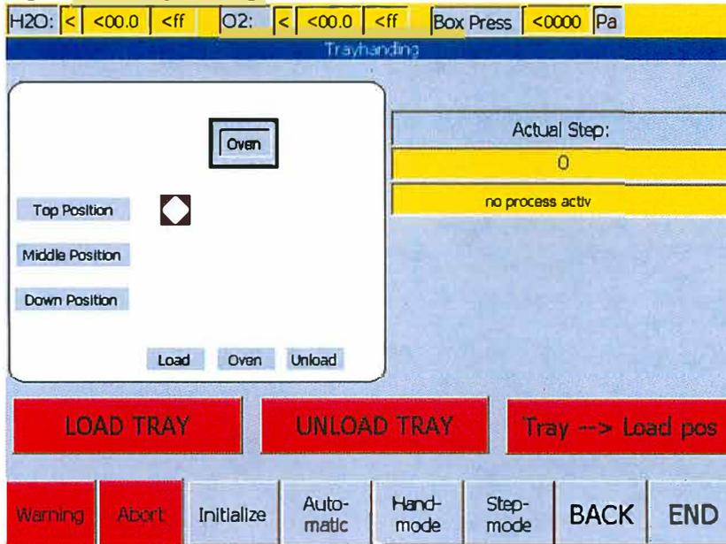
This screen also displays the position of the oven handler and the gripper. The yellow status field displays the current process step.
