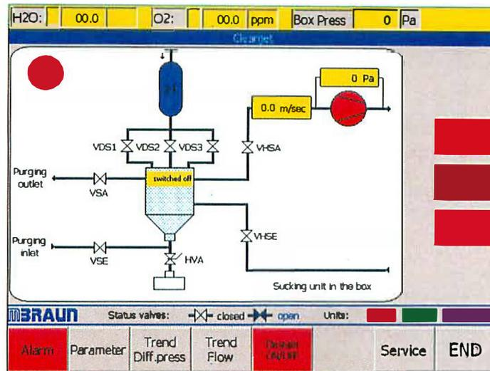
The main screen displays an overview of the **Clean-JET** system.
