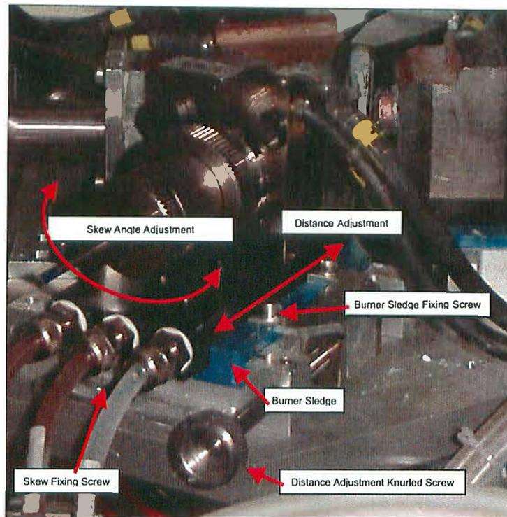
Fig. 15 : Plasma burner skew and distance alignment
