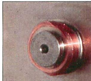
Fig. 13 : Correct position of cathode tip
