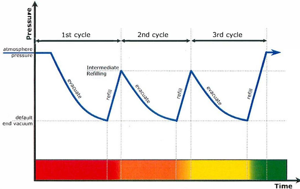
The diagram above shows how the intermediate refilling affects the atmosphere within the antechamber.
