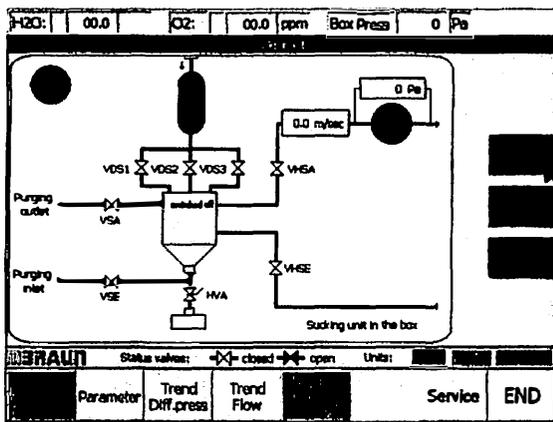
When the filter is exhausted there would be an increase in the differential pressure over the filter. If this difference pressure exceeds the setpoint "Maximum pressure filter" a warning will given on the Alarm/Warning Screen. This warning will indicate that the filter may require a cleaning process.
