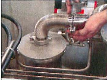
Detach clamp from the flange that connects the Safety Filter's flexible hose to the Main filter inlet pipe. (this pipe usually runs to the top of the Clean-JET cabinet in order to connect to the filter head).
