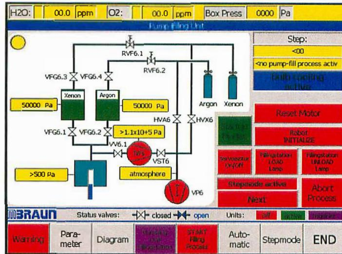
Fig. 4 : Pump Filling Unit screen
