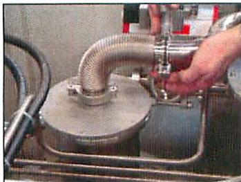
Replace the centering ring and O-ring seal, and re-clamp the flange connection.
