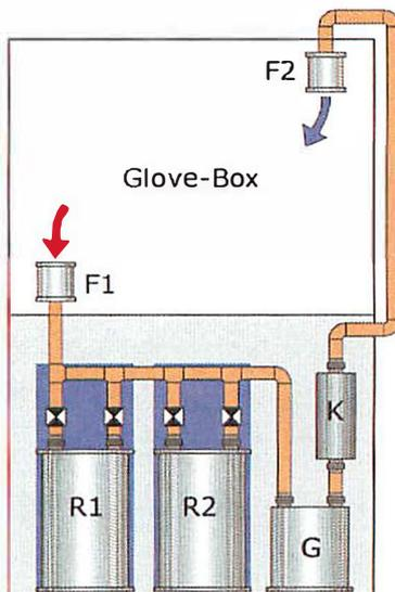
The diagram shows the gas flow in the circulation mode:
