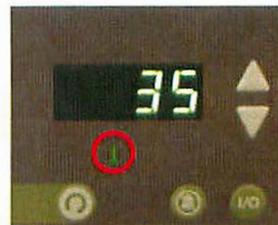
To change the values of parameters use the up/down keys. To set the new value press the menu/display key
