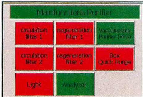
Selecting the Circulation Filter button a further time will switch off the circulation over the first purifier column.
