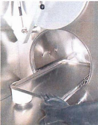
**After execution of the evacuation/refill cycles:** Opening and closing of the antechamber door inside the box is done in the same way as described for the outer door.
