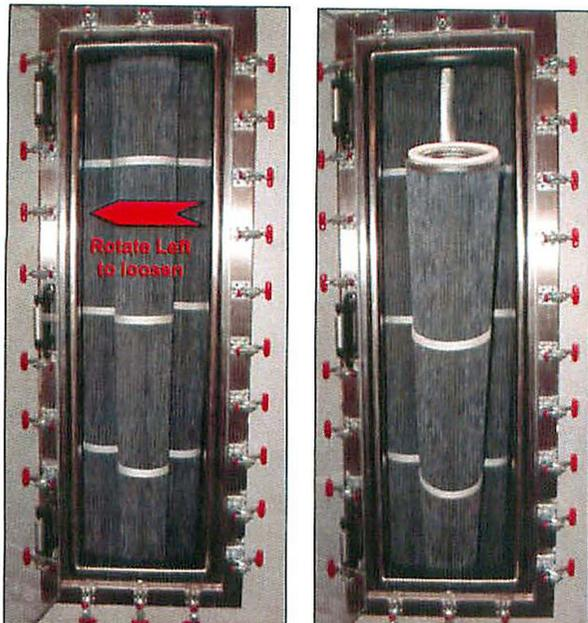
Remove the foremost filter by rotating it to the left, support the filter by holding the upper strap.
