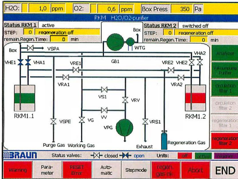
On the right-hand side of the screen are found the buttons for controlling the RKM and below are those for screen branching and for the functions.
