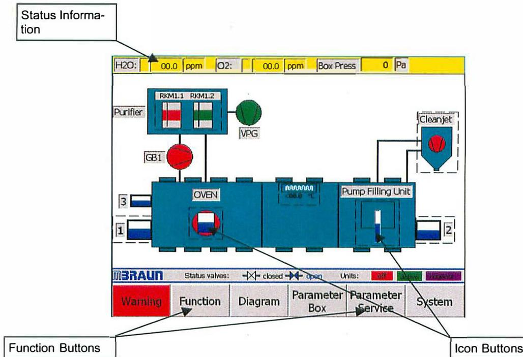
The Diagram above shows a typical "Start Screen". The various icons will change depending on the system chosen.
