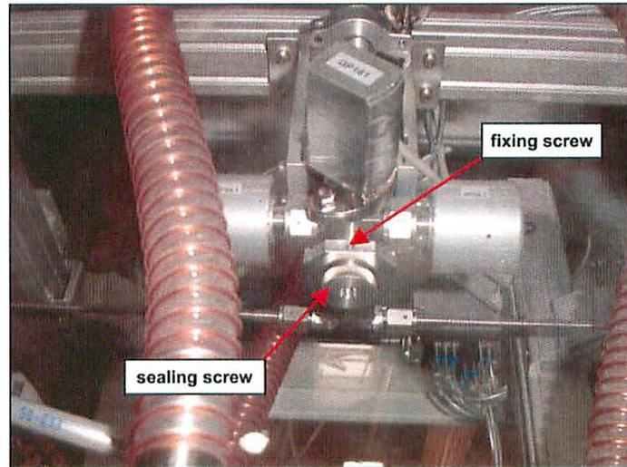
3. Remove the sealing screw by turning it counter-clockwise, the bushing is loose inside the screw.
