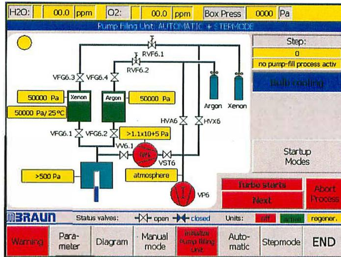
Fig. 3 : Pump Filling Unit screen
