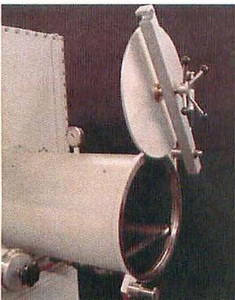
The antechamber door is held by the spring mechanism. It stays in the position (see picture).
