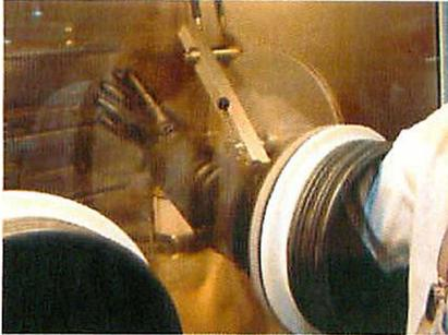
Check that the glove is orientated correctly and replace with new O-rings.
