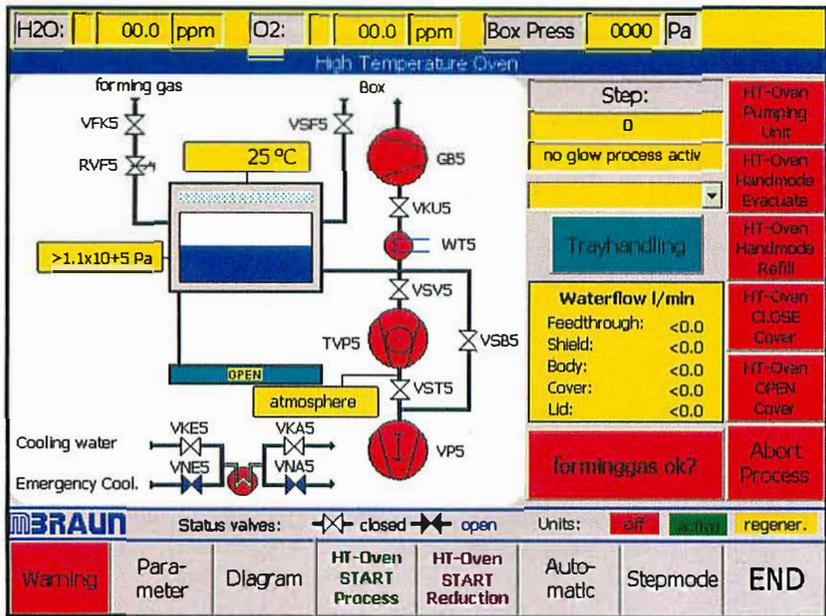
The picture shows the schematic diagram of the process oven. The yellow status fields show various observed values or process steps.
