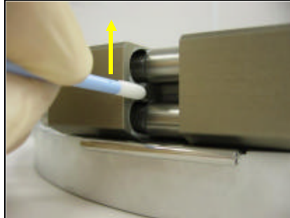
[Figure 6-H, Clean off any excess grease with a swab]
