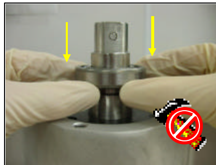
[Figure 9-E, Install the Bearing straight on the Shaft]
