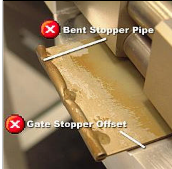
[Figure 5-G, Check for Gate Stopper Damage]
