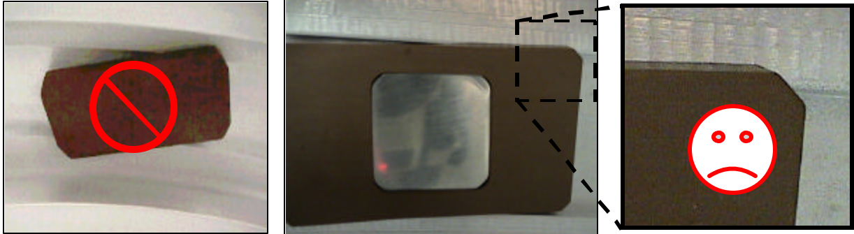
[Figure 11-E, Incorrect (diagonal) installation of the hard stop]
