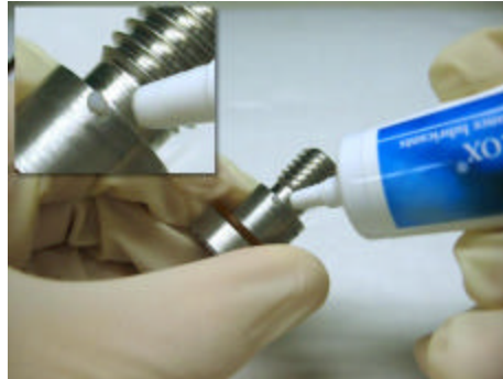
[Figure 12-A, Spread ¼ bead on the Power Bolt shoulder]
