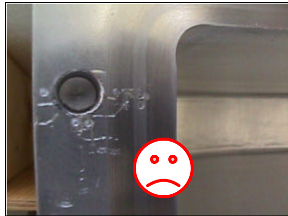
[Figure 12-F, Avoid damage to the Bonnet sealing surface]
