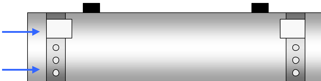
[Figure 14-C, Push the sensor toward the center until the LED on the 9V test circuit illuminates]
