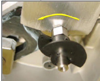
[Figure 8-C, Unscrew the “Flag Pole” with the Nor-Cal “Super Wrench”]
