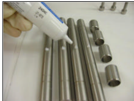
[Figure 6-F, Add 1 bead of grease to each Holder and spread evenly]
