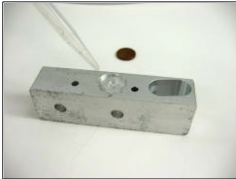
[Figure 6-I, Add a drop of DI water and install the Slide Pads]
