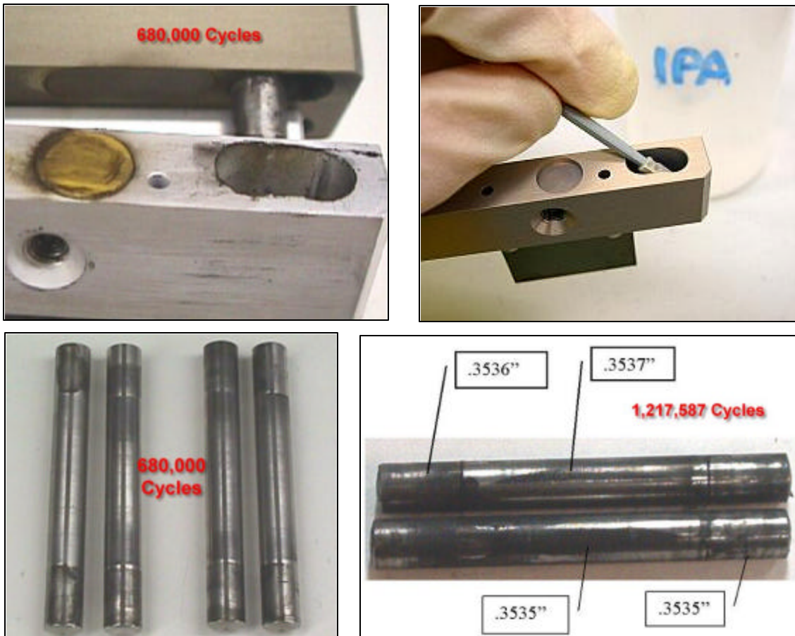
[Figure 5-I, Examples of high-cycle Holder and Roller wear]
