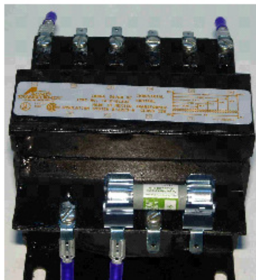
460/480V Setting (Factory setting for high voltage models)
