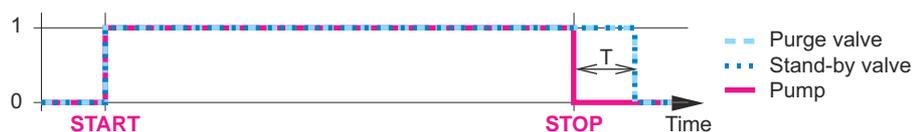
**ENABLED** The **stand-by (4)** and **purge (3)** valves open/close simultaneously following a **PURGE** command independent of the pump being started/stopped:
