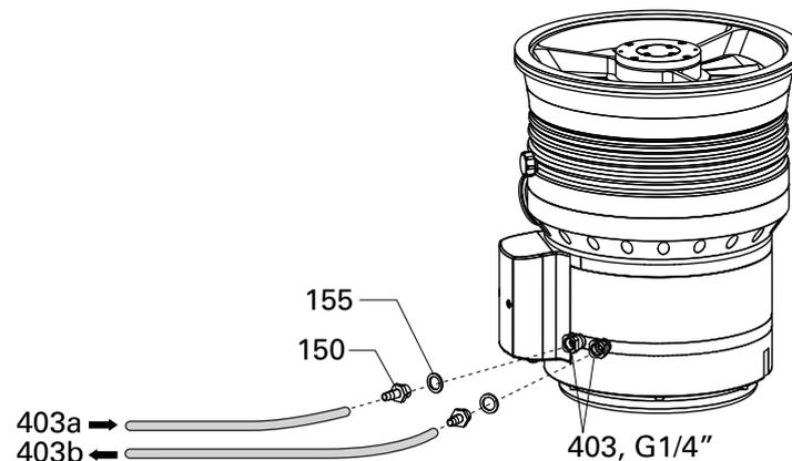
**Fig. 15: Connecting the cooling water**
