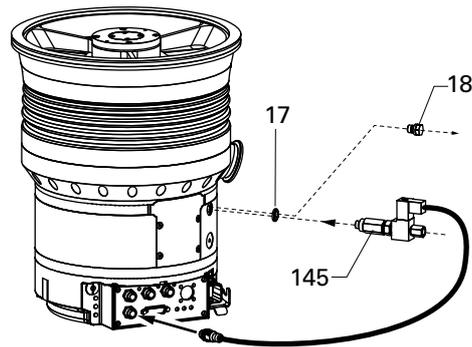
**Fig. 13: Connecting the sealing gas valve**
