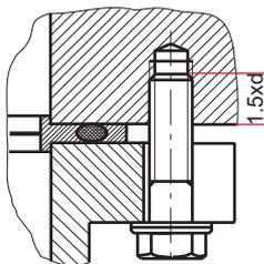
The connection types for installation of ISO-F to ISO-F flange are "hex screw and threaded hole," "stud screw and threaded hole," and "stud screw and through hole".
