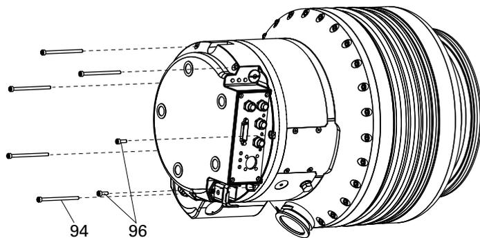
→ Tighten the electronic drive unit 13 with allen head screws 94 (5x) and 96 (2x).
