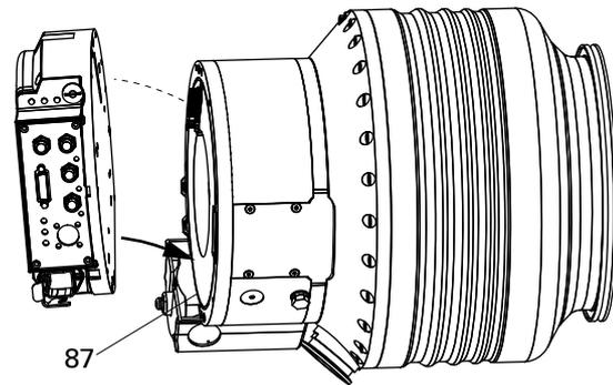
→ Fix the O-ring 87 in the groove of the pump bottom part, if necessary. Ensure correct seating!
