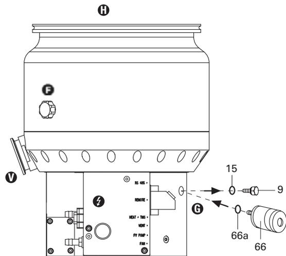
Please refer to Operating Instructions PM 0229 BN for details on installing the sealing gas valve and adjusting the sealing gas flow.
