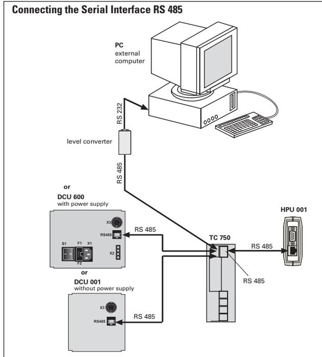
The serial interface is galvanically and safely separated from the maximum supply voltage from the TC 750.
