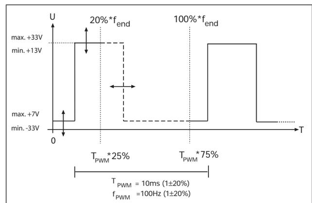
If no signal is present the pump runs up to its final rotation speed.
