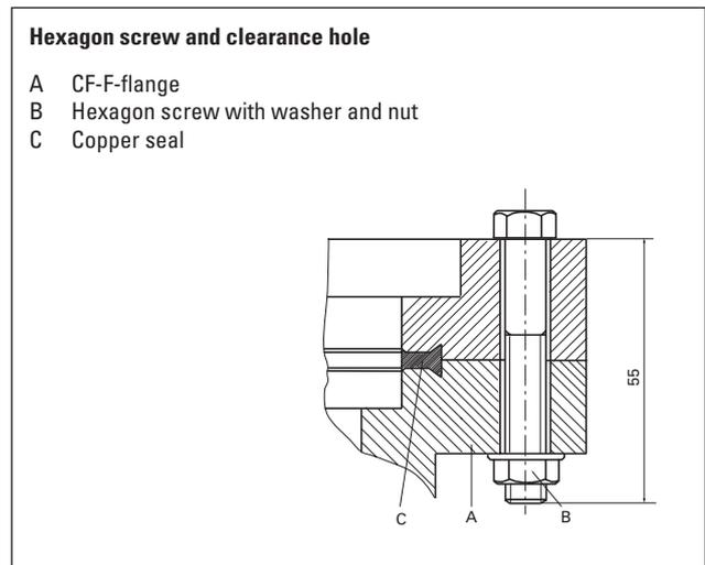
The components for installing to an CF-F flange are to be ordered under the following numbers:
