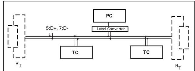
All units connected to the bus must have differing serial interface addresses (parameter 797). The group address of the TC 750 is 960.
