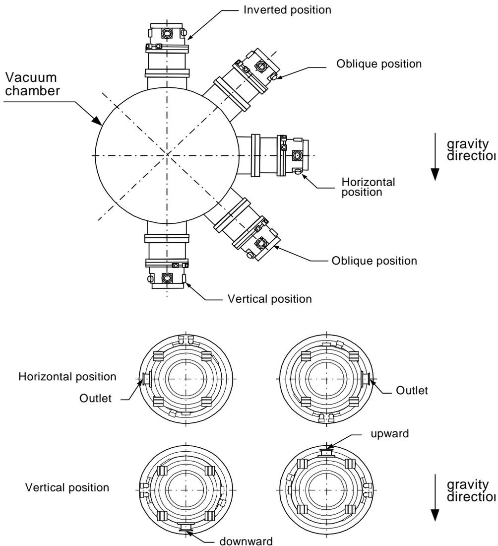
The outlet of the magnetic bearing turbomolecular pump should face horizontally or vertically when installing horizontally.
