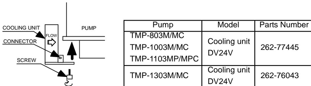
**Fig. 1 How to Change the Cooling Fan Unit**
