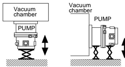
**Fig. 5-3 Lifting Method**
