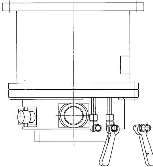
**Fig. 5-7 Cooling Water Piping Connection**
