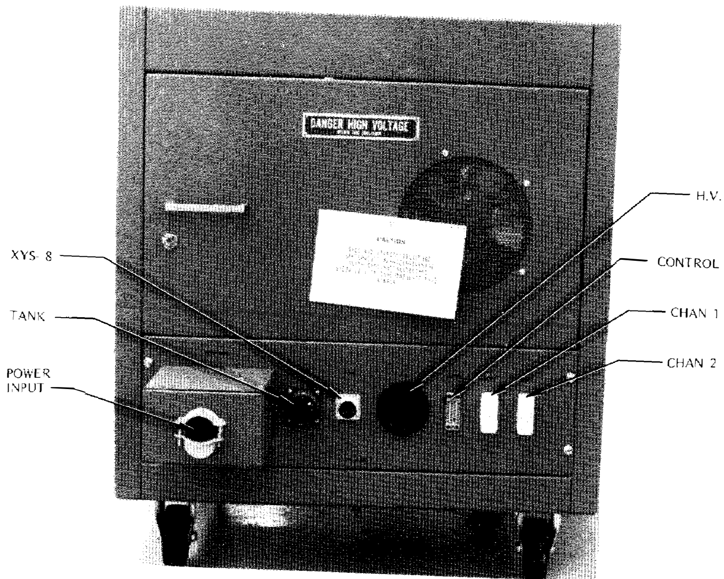
Figure 2-6. CV-8 A and B power supply (rear view).
