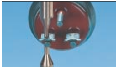
Weld electrical terminals to solid wire leads
