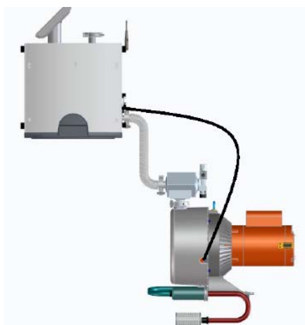
Figure 1-14 Bench Mount Leak Detector with External TS620 Dry Scroll Pump, Model G8612
