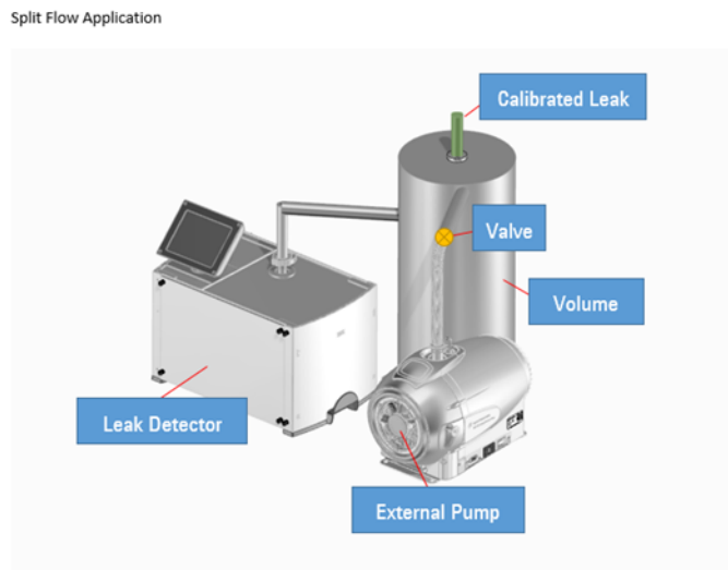
Figure 5-12 Split Flow Application
