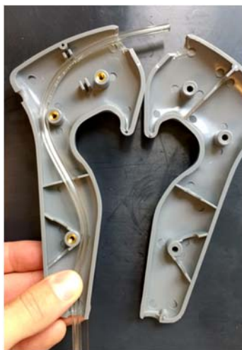
Figure 5-21 Re-purposing a Power Probe for Thin Hose Without a Regulator
