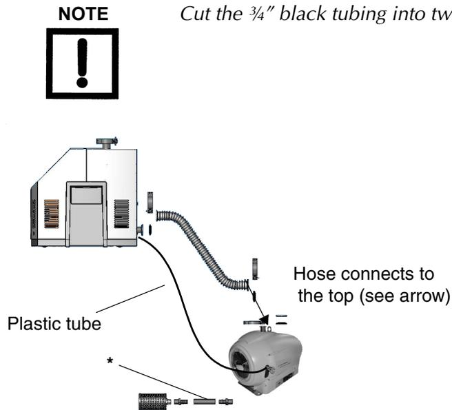
**Figure 1-12 Bench Mount Leak Detector with External IDP-15 Dry Scroll Pump, Model VS BD15**
