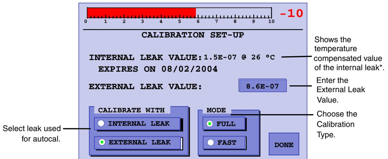
**Figure 2-8 Calibration Set-Up**
