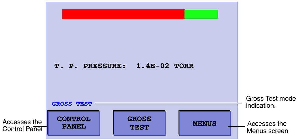
**Figure 2-3 Gross Test Screen**
