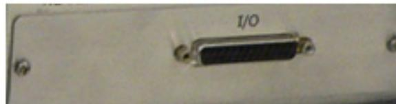
**Figure 1-16** Optional I/O PCB Rear Panel
