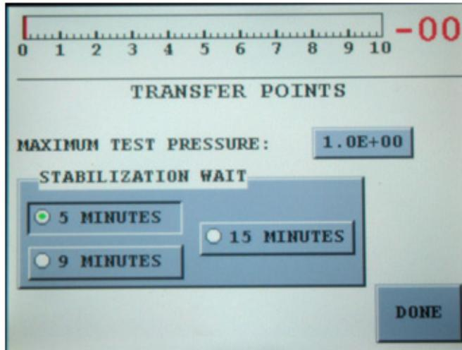
**Figure 2-14 Transfer Points with Stabilization Wait Timer**
