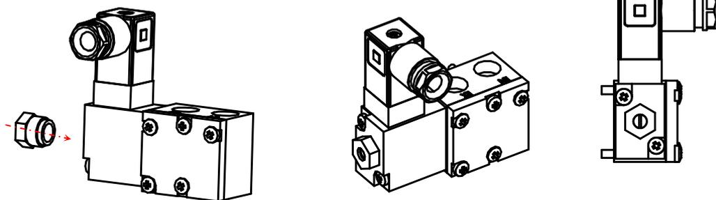
Push and rotate in lockable: valve opens
