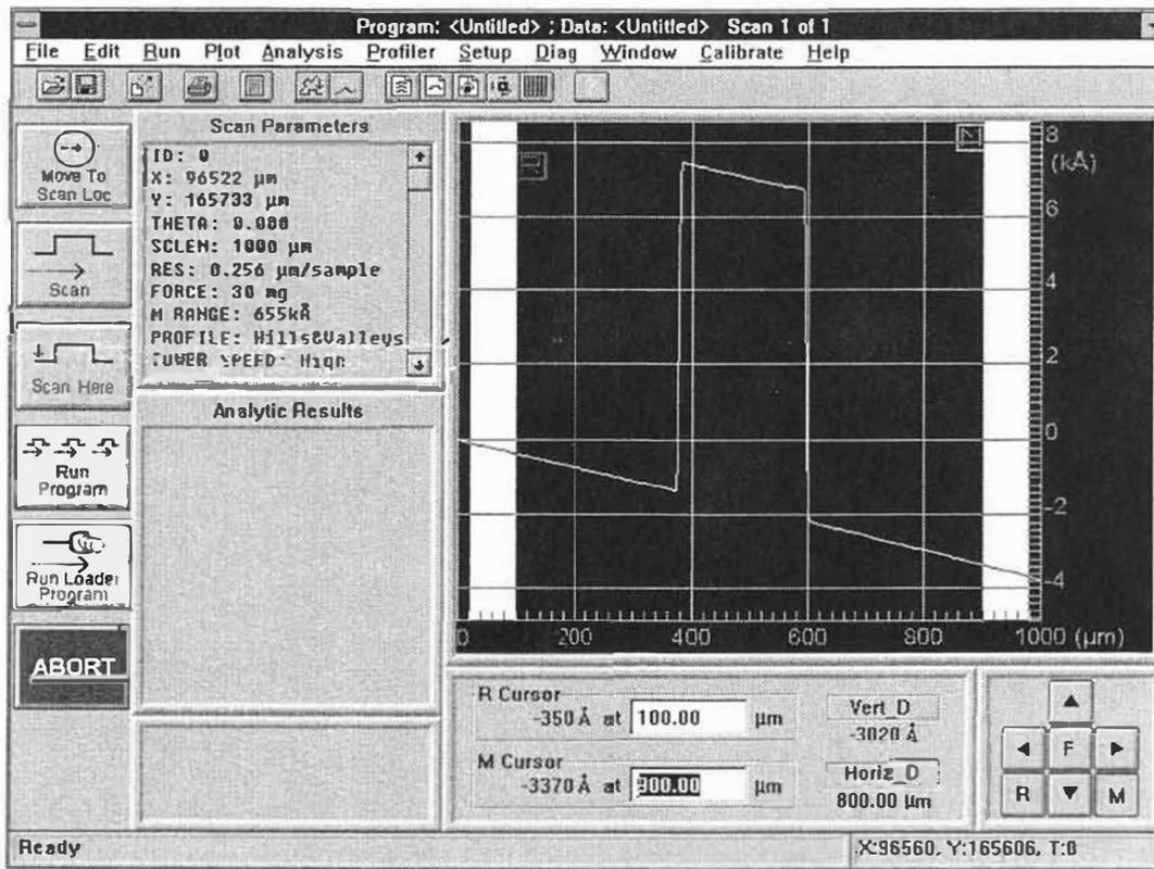
Figure 4-5. Setting the M Cursor at 900  $\mu\text{m}$
