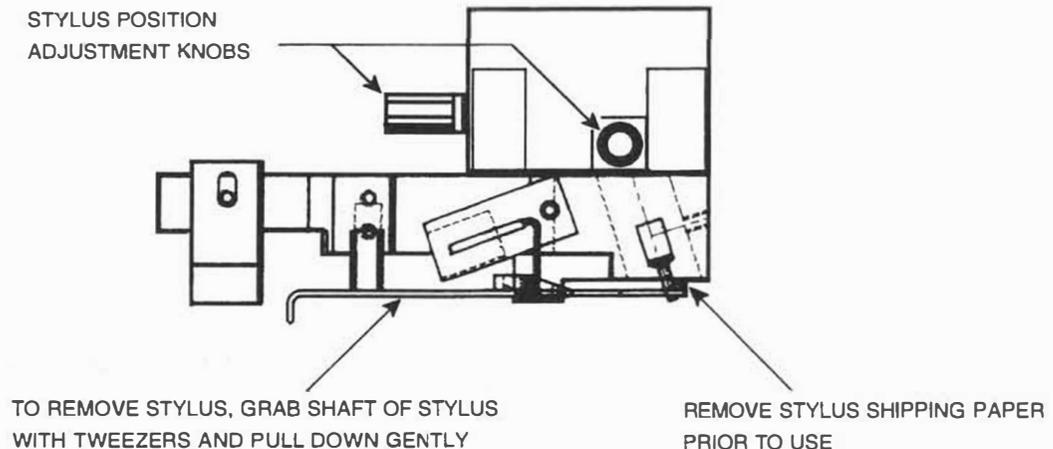
**Figure 10-11. Low Inertia Sensor Head**
