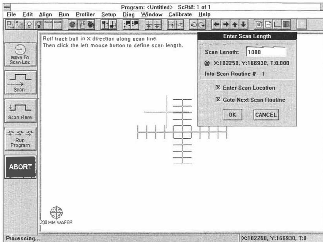
Figure 4-2. Entering 1000 Micron Scan Length into a Scan Routine
