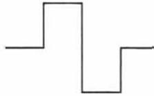
(Hills and Valleys) Provides 50% of the measurement range above the zero horizontal grid line and 50% below. Used in most applications, especially if the surface characteristics of the sample are not well known, or if the sample is out of level.
