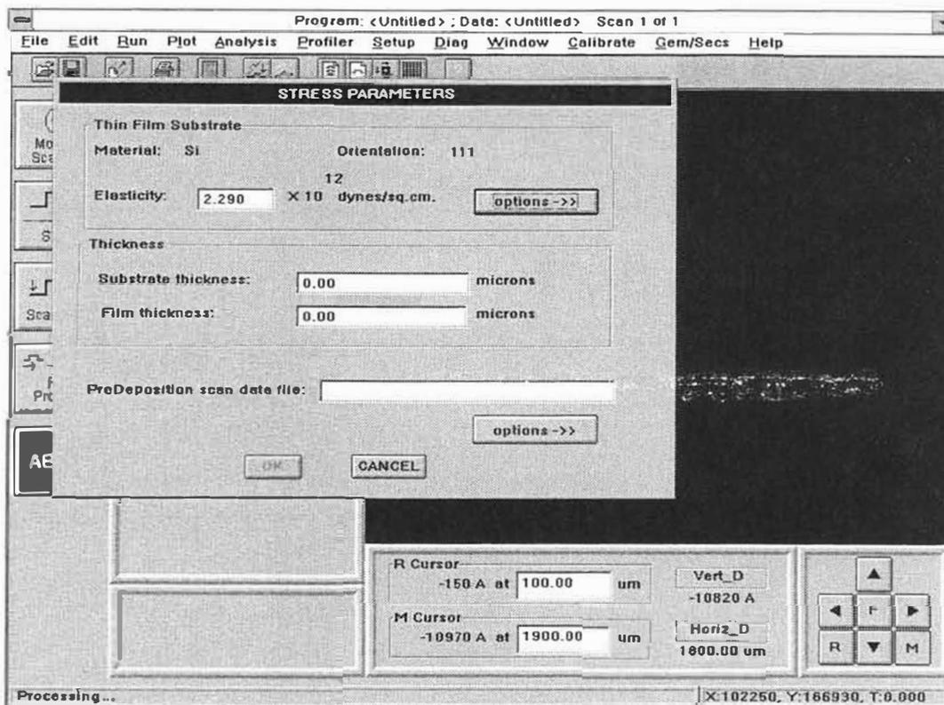
Figure B-2. Stress Measurement Dialog Box
