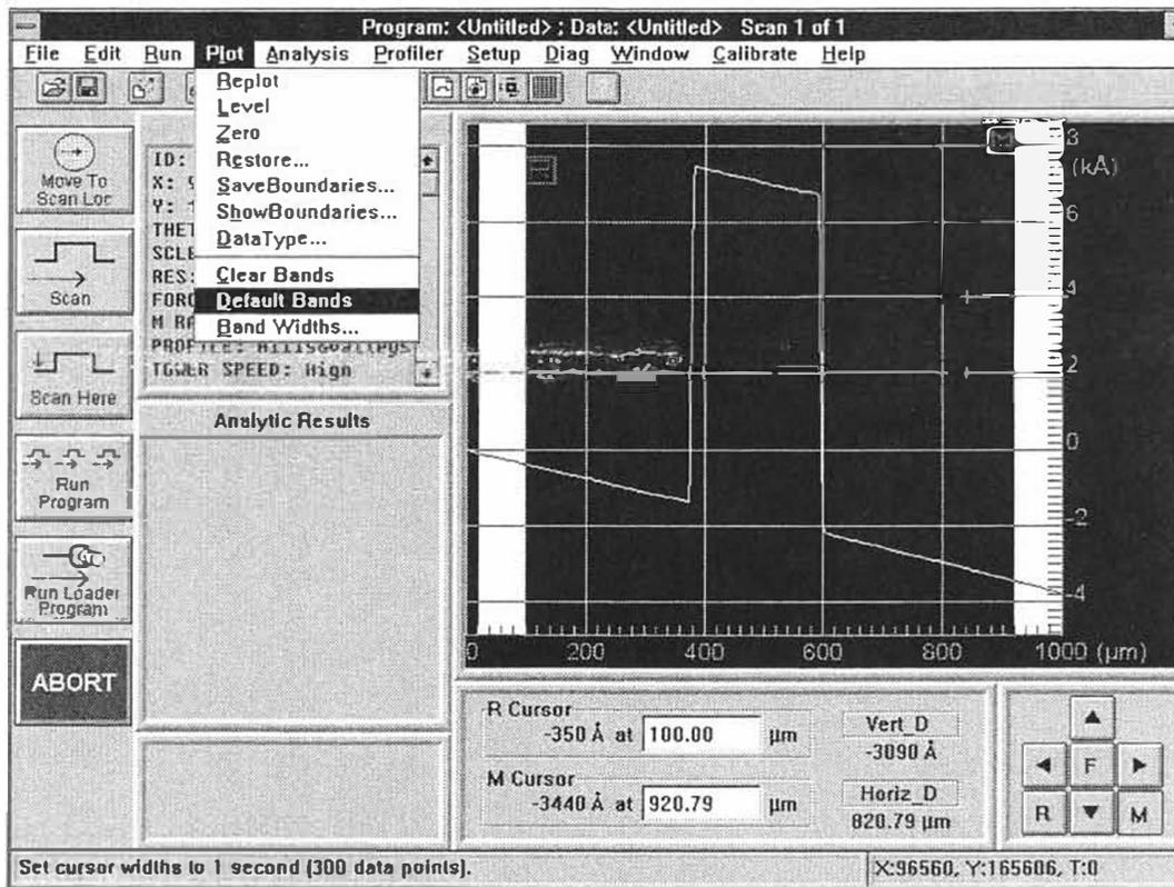
Figure 4-4. Setting the Default Cursor Band Widths
