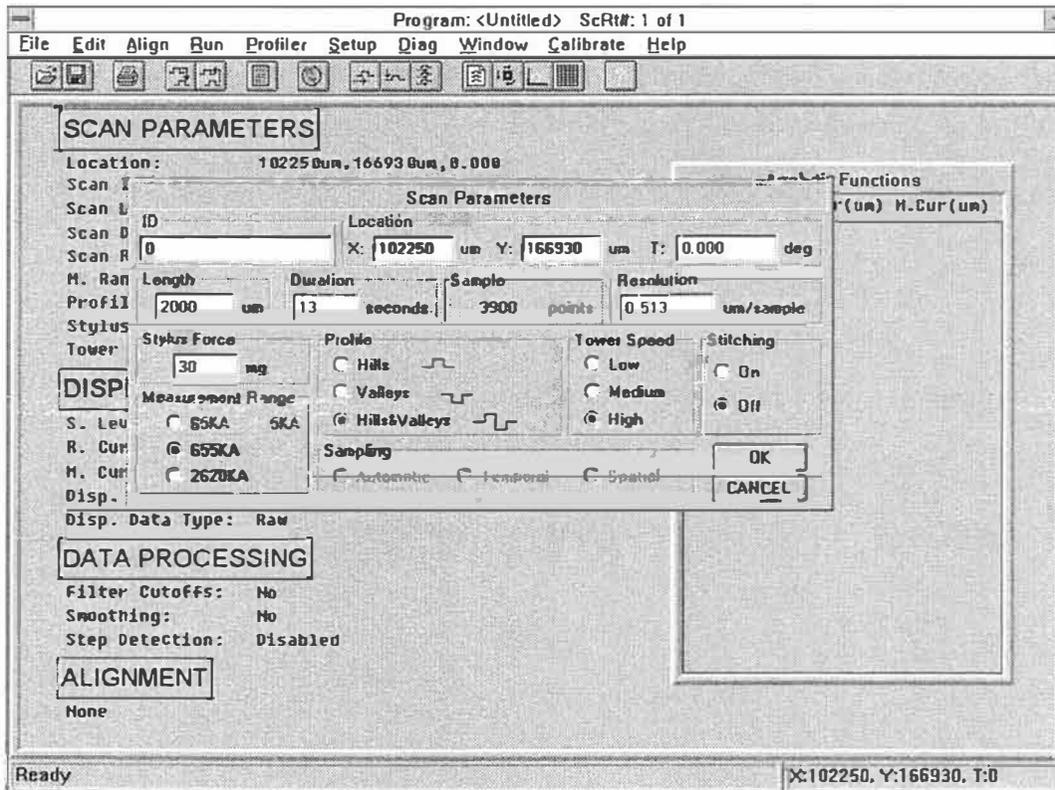
Figure 8-3. Measurement Range Parameter
