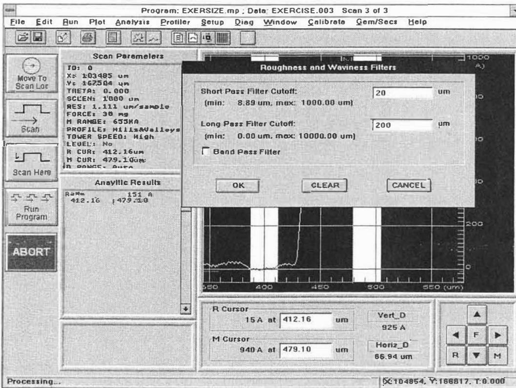
Figure 6-3. Roughness and Waviness Filter Dialog Box
