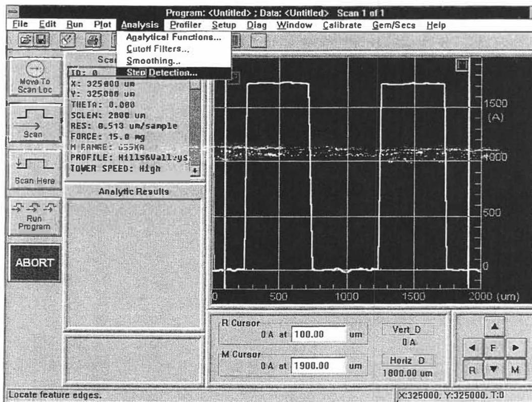
Figure E-3. Typical Scan of a Step
