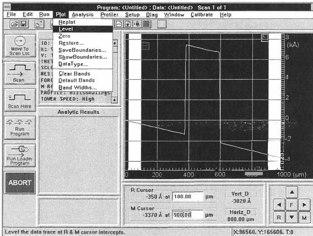
Figure 4-8. Cursor Positioning for Software Leveling
