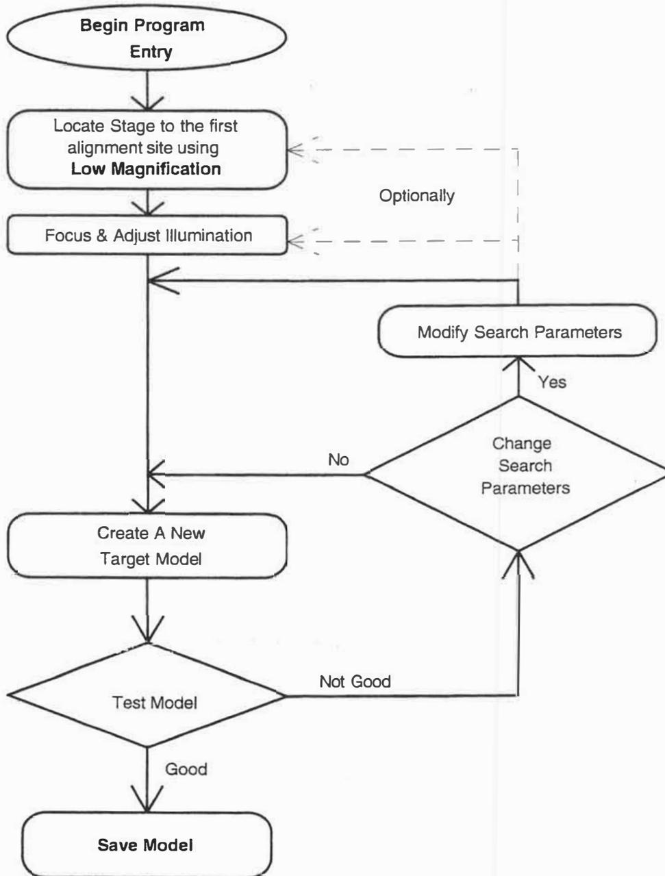
Figure F-1. First Alignment Location Flow Chart
