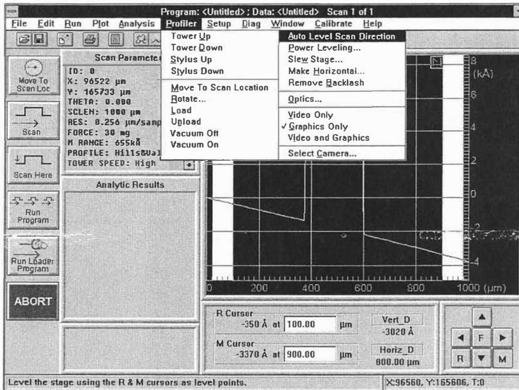
Figure 4-6. Auto Leveling of the Stage
