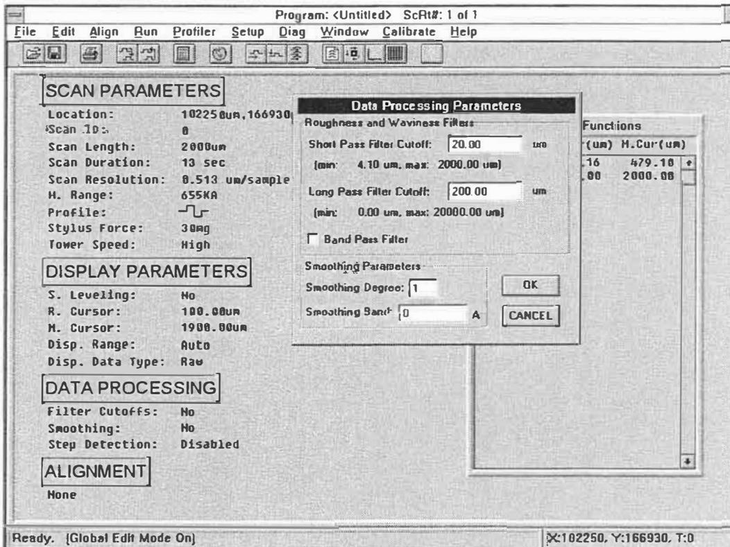
Figure 6-7. Filter Cutoffs Parameter
