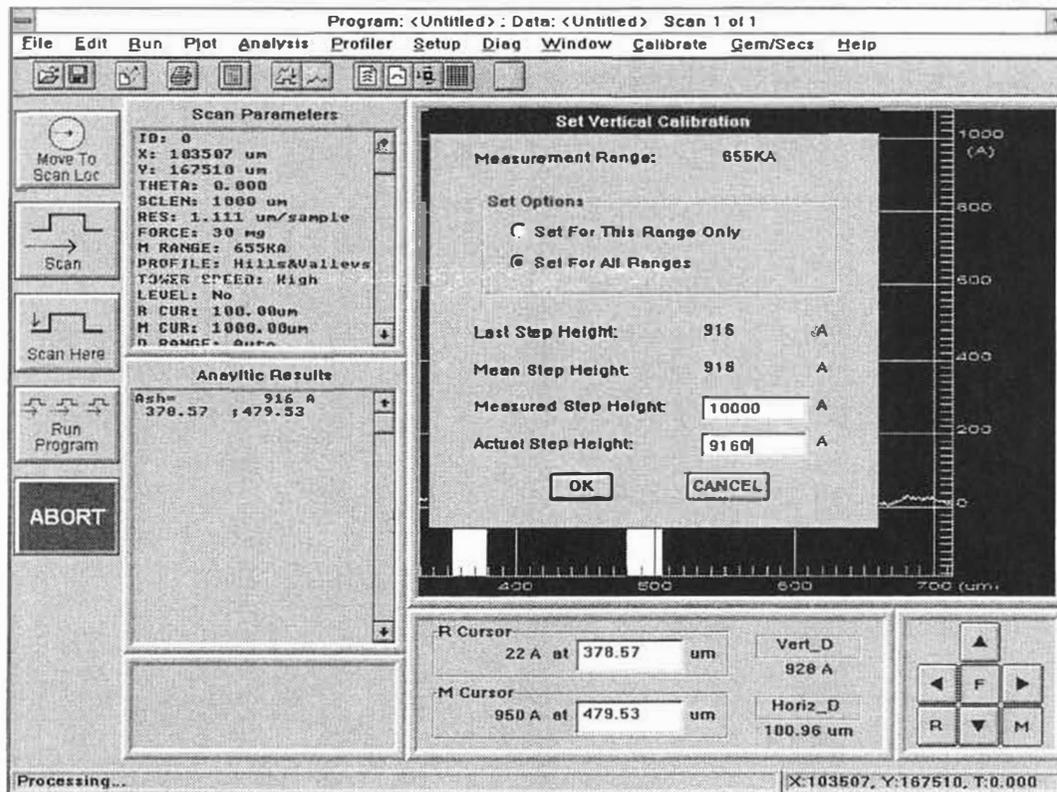
Figure 10-4. Set Vertical Calibration Dialog Box
