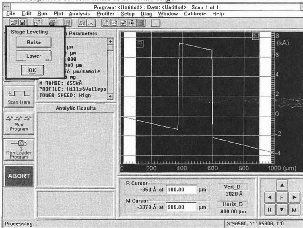
Figure 4-7. Stage Leveling Window
