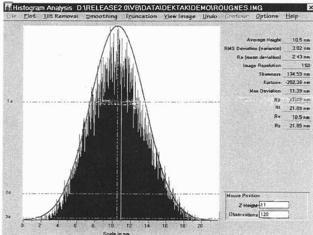
Figure D-10. - Histogram Analysis Window, Showing the Z Height Histogram Plot
