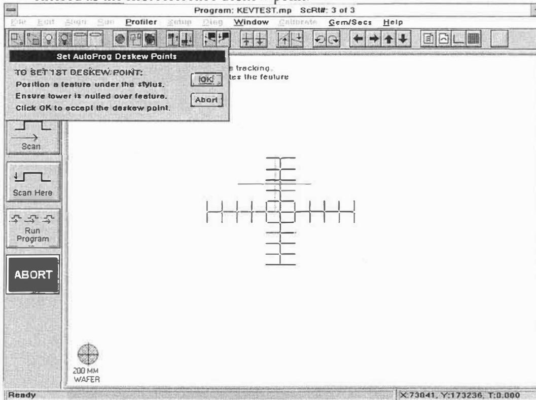
Figure 5-16. Setting the First Reference Deskew Point
