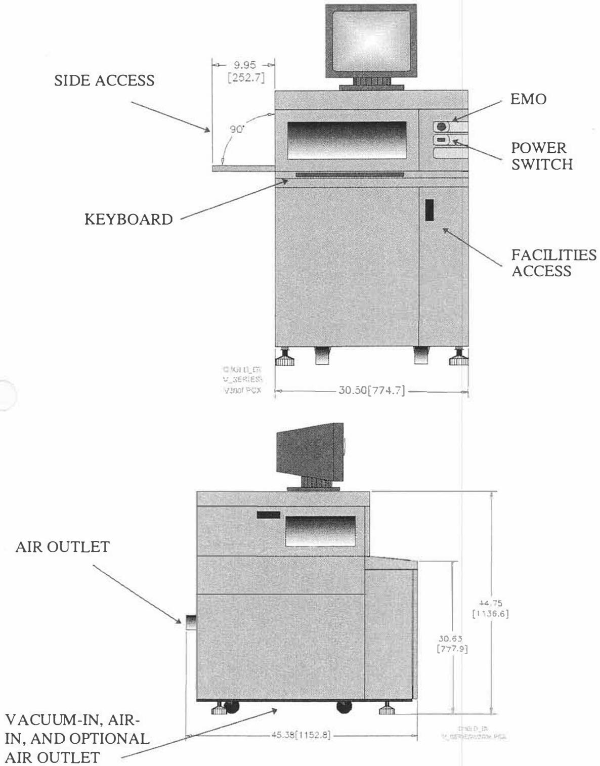
Figure 1-2. Physical Characteristics
