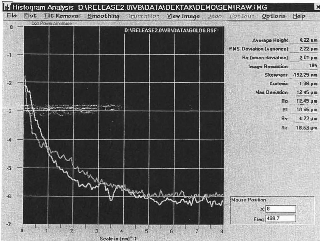
Figure D-11. Roughness Frequency Plot with Additional Roughness Parameters
