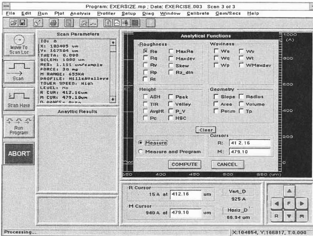
Figure 6-2. Roughness Functions Window
