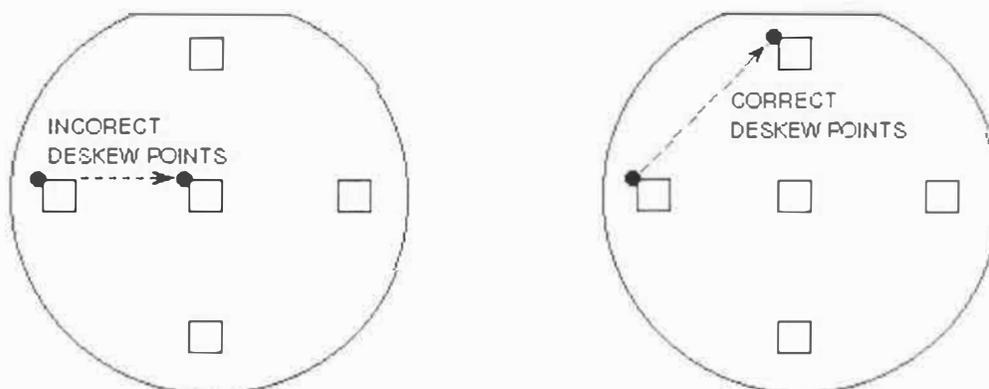
**Figure 5-15. Establishing Deskew Points at a Diagonal**
