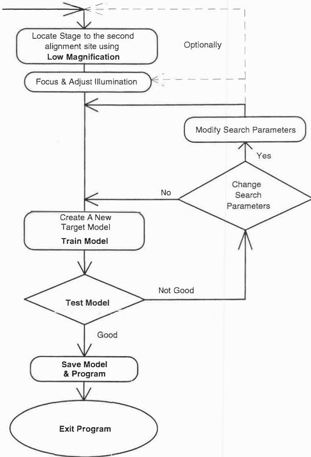
Figure F-2. Second Alignment Location Flow Chart
