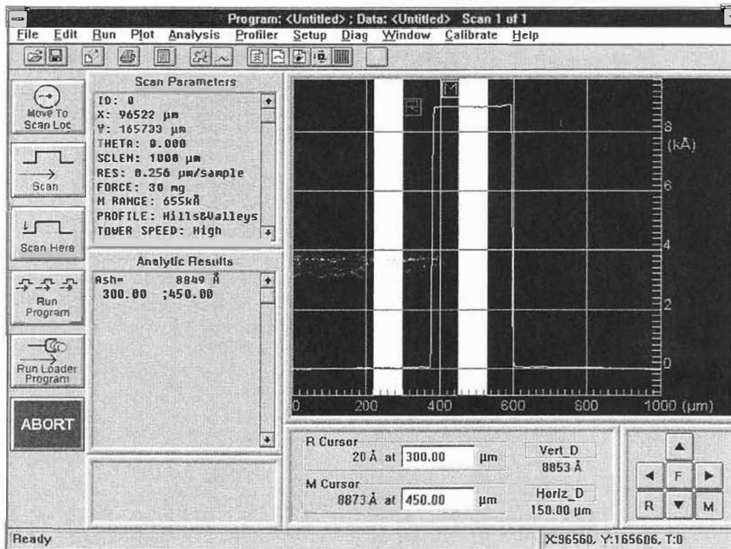
Figure 4-10. Step Height Measurement
