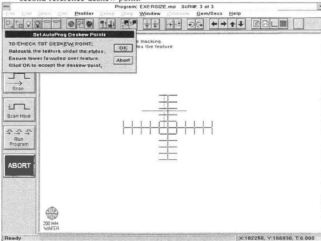
Figure 5-18. Checking the 1st Actual Deskew Point
