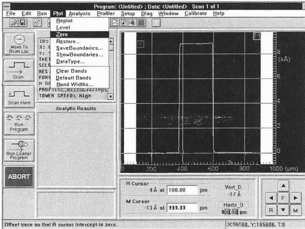
Figure 4-9. Setting the Zero Point
