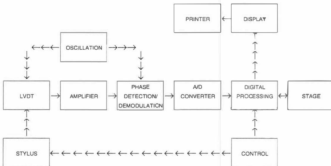
Figure 2-1. Block Diagram of DEKTAK V 200-Si Architecture
