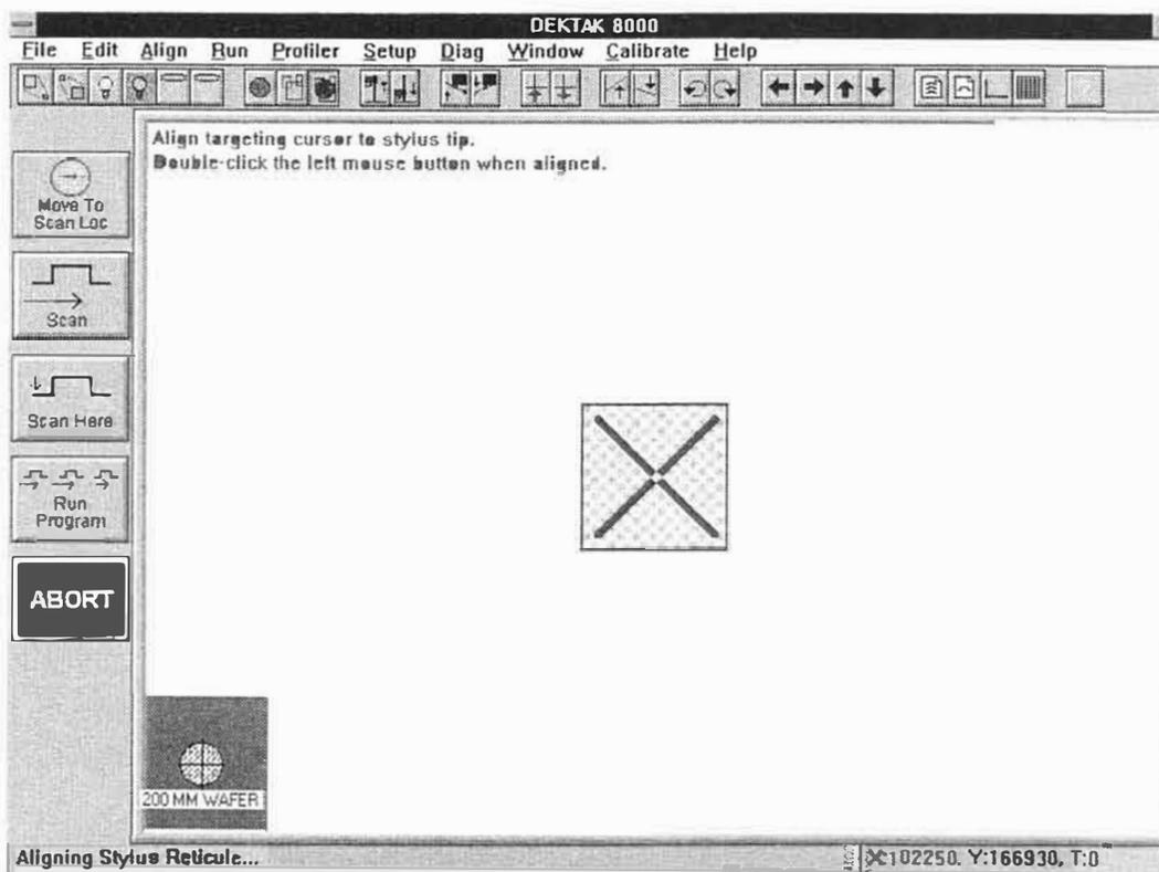
Figure 3-10. Stylus Reticule Alignment
