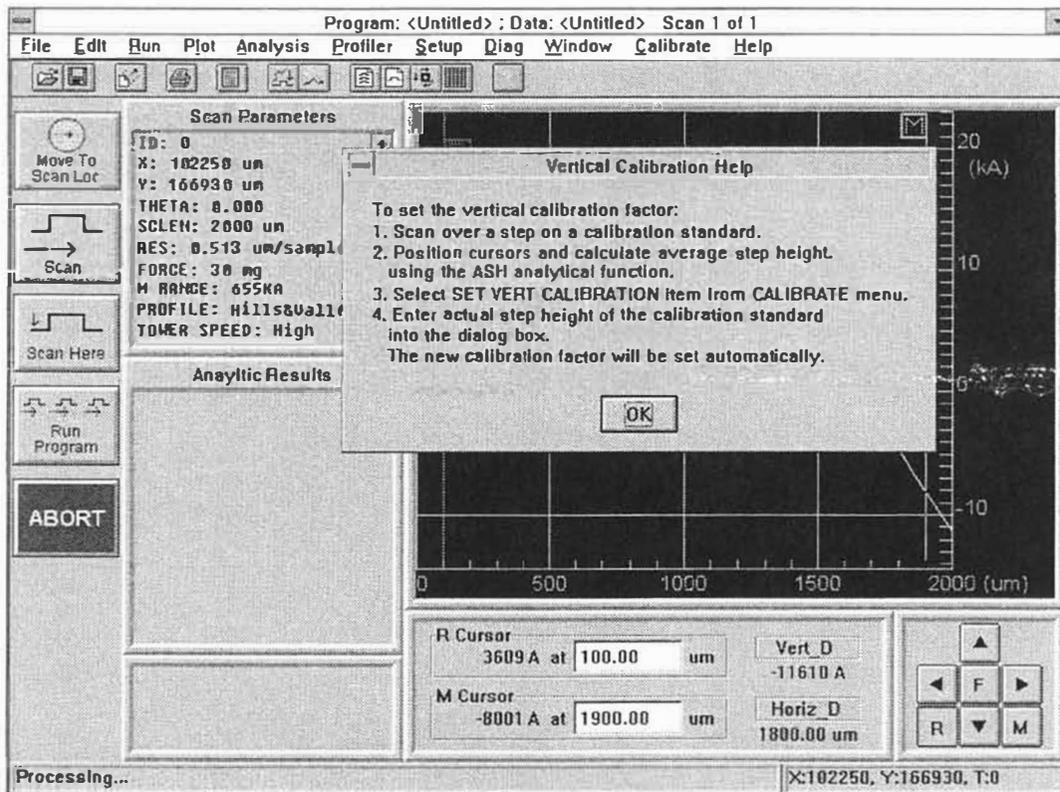
Figure 10-1. Vertical Calibration Help Window
