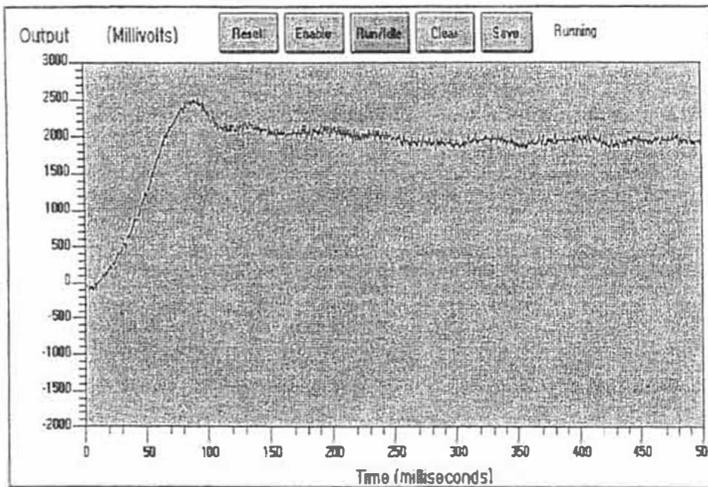
Note that the start-up voltage is about 2.5 V on this example. A properly aligned axis should have no more than 3 V start-up voltage. The excursions after the voltage settles should not exceed  $\pm 0.3V$ . Loosen the mounting hardware and repeat motion until performance shown to the right is attained.
