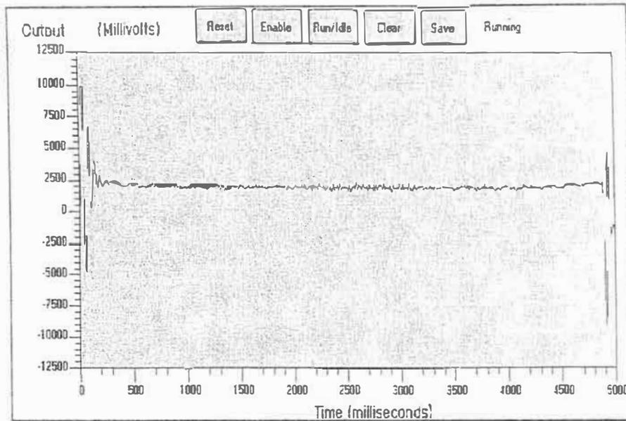
Voltage excursion after settling should not exceed +/- 1V. If this occurs, stop motion, loosen mounting software, and restart motion until hardware has been adjusted to sufficiently reduce the excursions.
