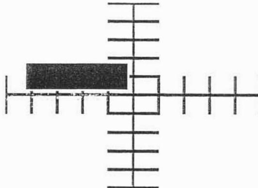
**Figure 3.1.4.2 - Suggested Positioning of Reticule With Respect To Feature**
