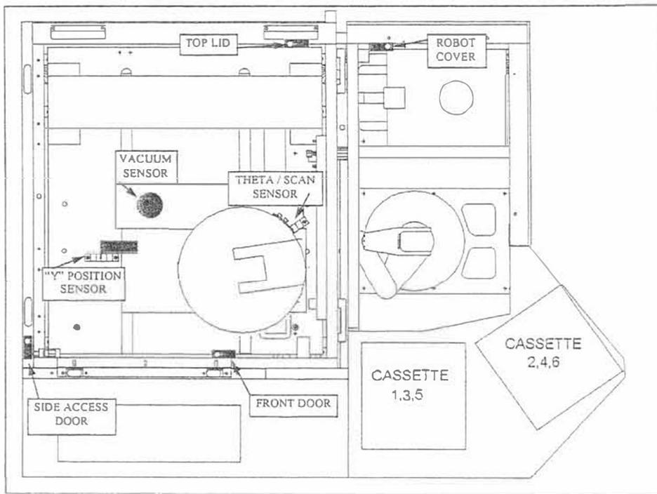
Figure 3: Sensor and interlock switch locations
