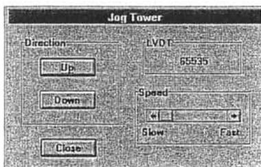
Adjust the position of the tower until the center 1/3 of the screen is in focus. To determine the best position, locate some vertical features on the display (e.g. closely-spaced lines), then position the tower until their center portion appears to be focused.
