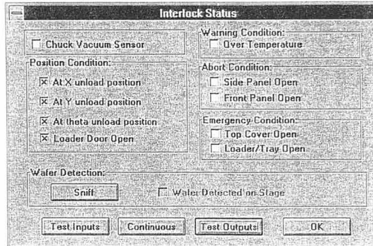
If the indications do not match the window above, adjust the sensors for the scan, Y, and theta (stage) unload position sensors per the instructions below as appropriate:
